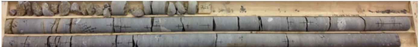
Borehole WC2 Elevation 229.3 m to 226.0 m
