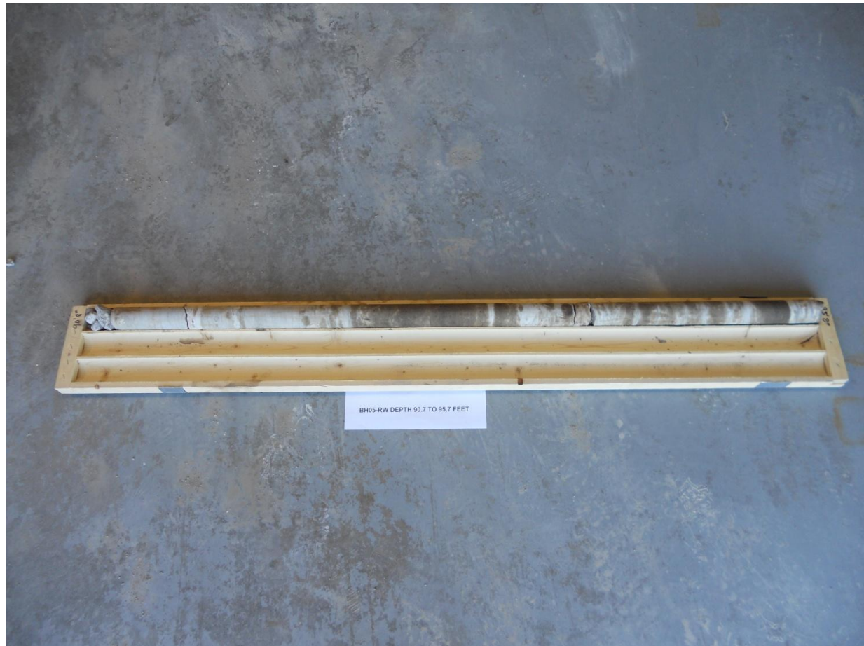
Photograph F-4: Borehole B05-RW – Rock Core Elevation 154.8 to 153.3 m
