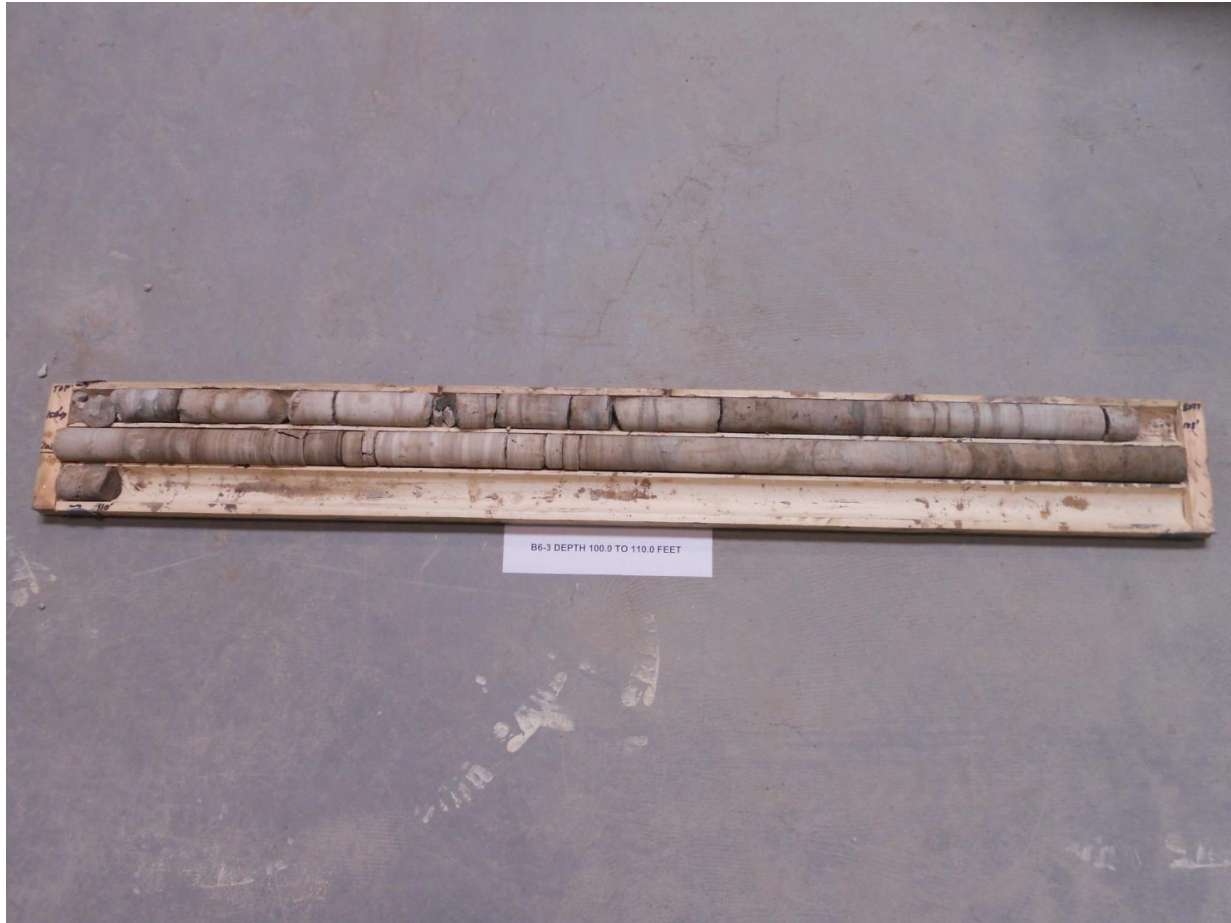
Photograph F-13: Borehole B6-3 – Rock Core Elevation 149.9 to 146.9 m
