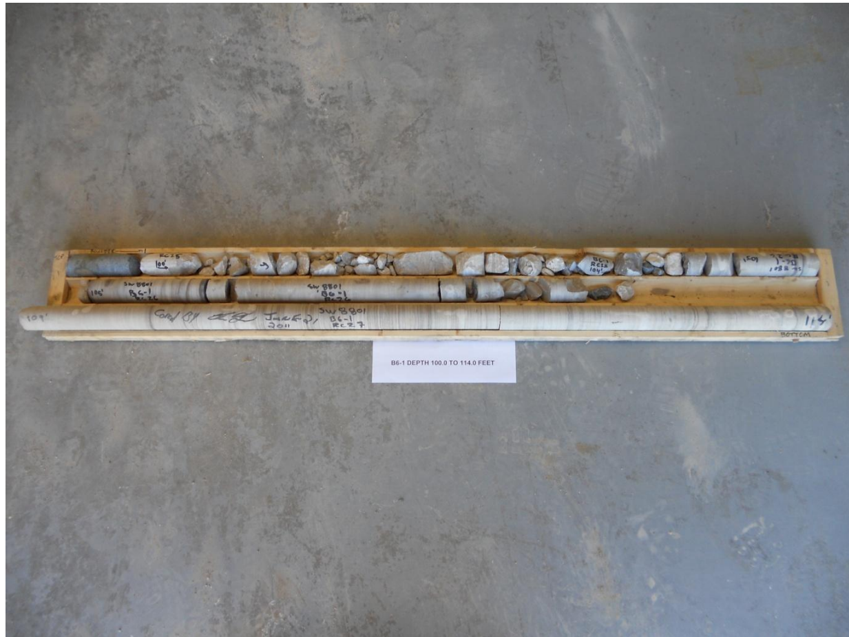
Photograph F-11: Borehole B6-1 – Rock Core Elevation 149.7 to 145.5 m
