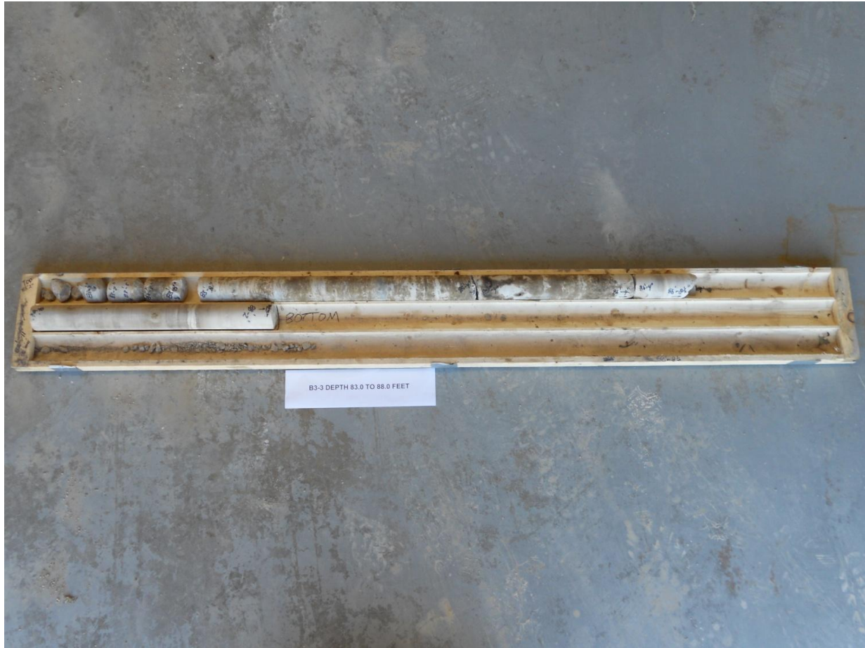
Photograph F-9: Borehole B3-3 – Rock Core Elevation 153.7 to 152.2 m
