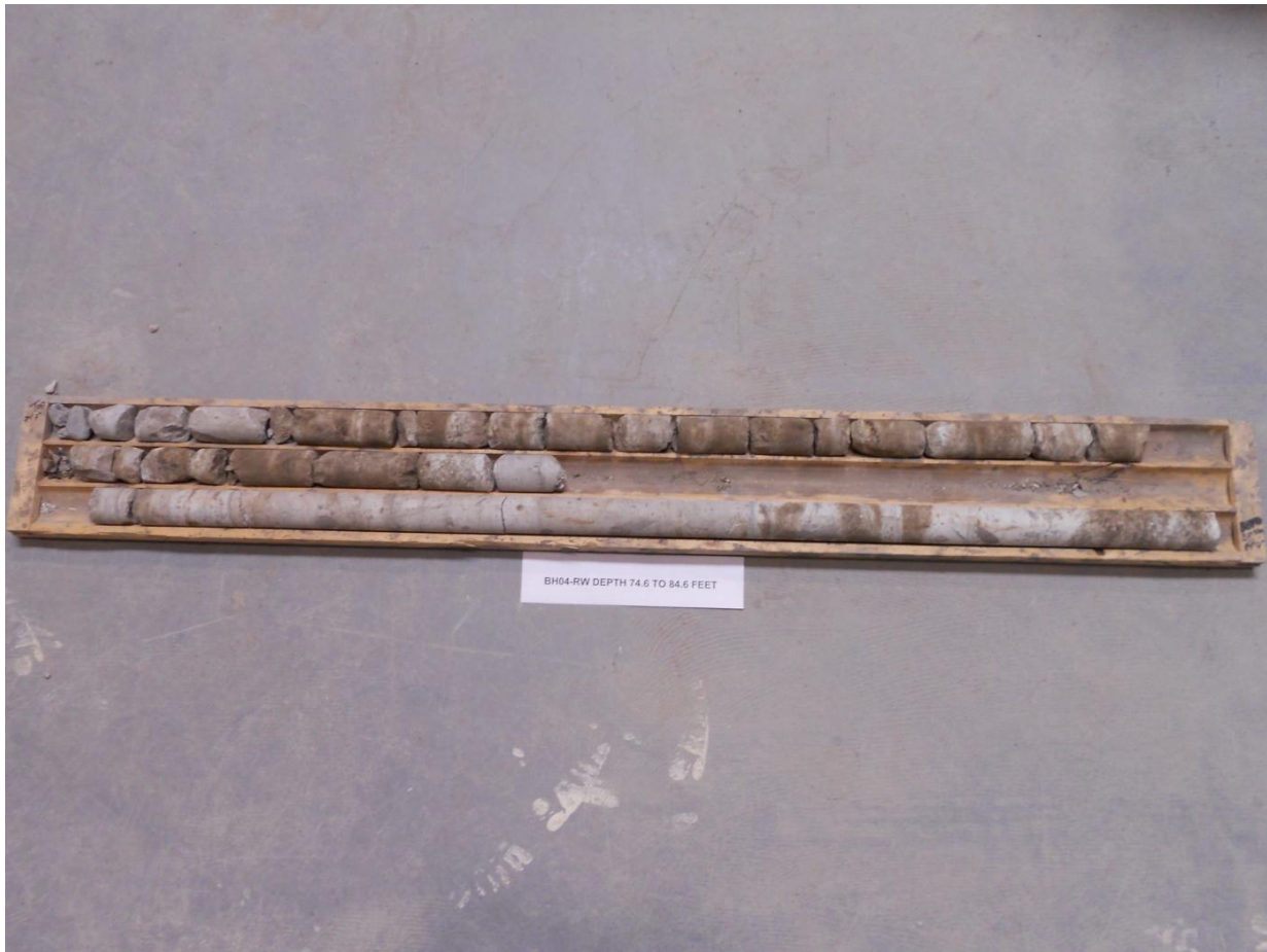
Photograph F-3: Borehole B04-RW – Rock Core Elevation 155.6 to 152.5 m
