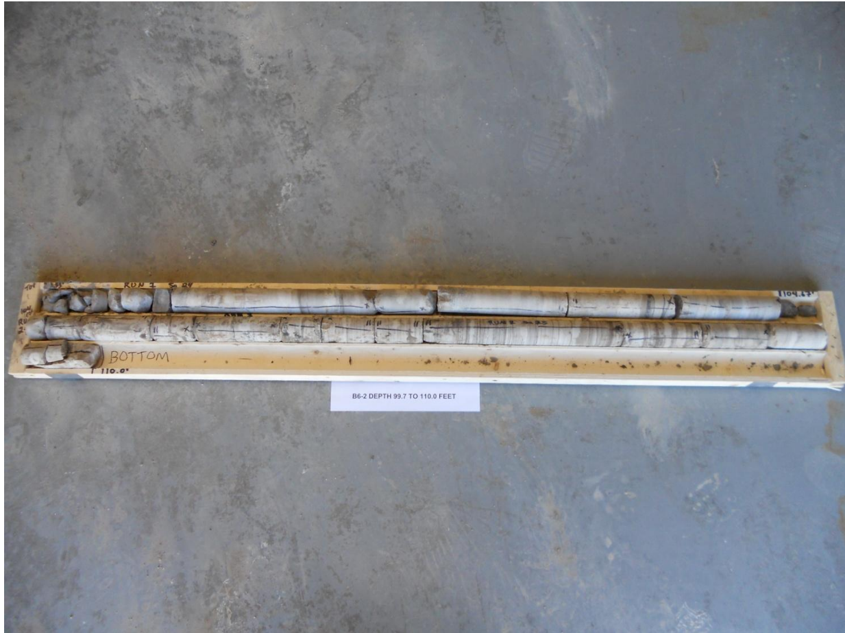
Photograph F-12: Borehole B6-2 – Rock Core Elevation 149.7 to 146.6 m
