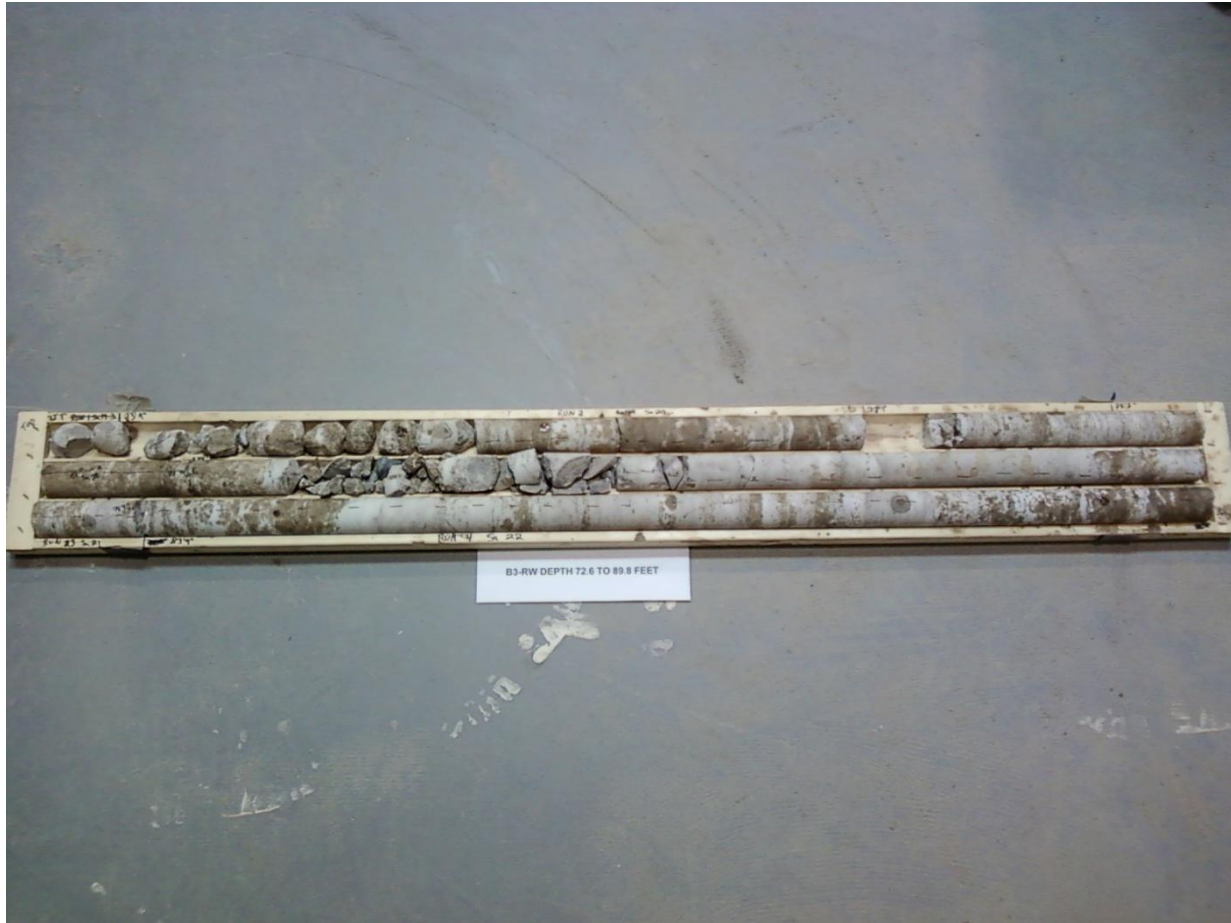
Photograph F-2: Borehole B03-RW – Rock Core Elevation 156.5 to 151.2 m
