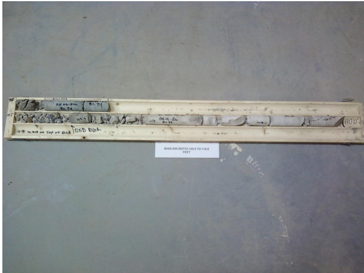
Photograph F-5: Borehole B06-RW – Rock Core Elevation 148.8 to 147.3 m
