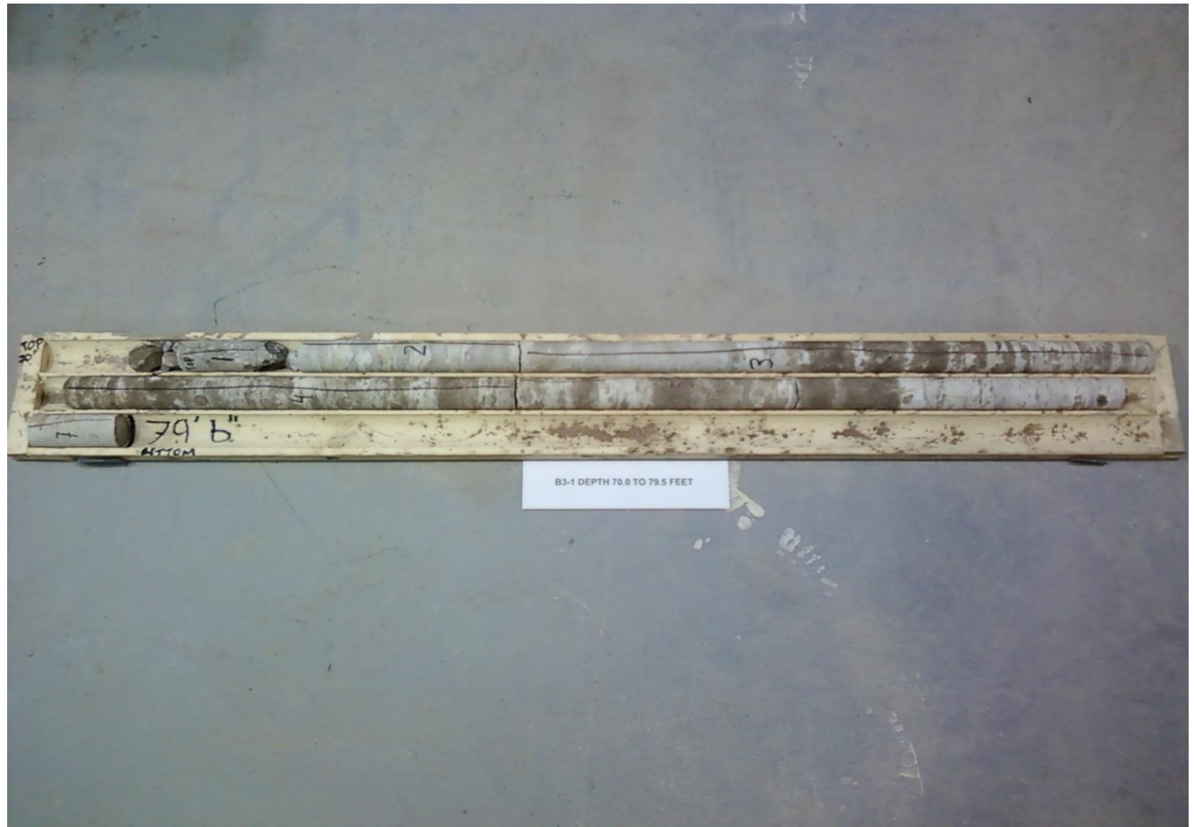
Photograph F-7: Borehole B3-1 – Rock Core Elevation 157.6 to 154.7 m
