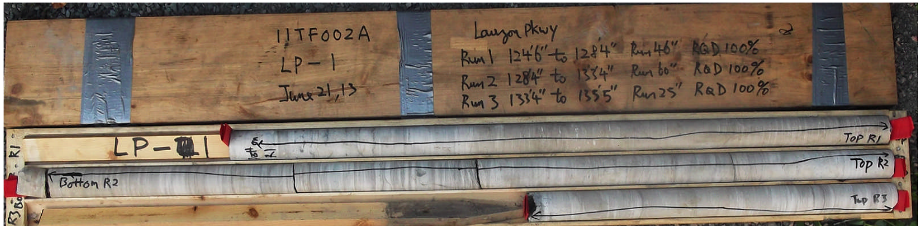
Photograph 1: Core retrieved from borehole LP-1. Rock cores 1 to 3 from 37.9 to 41.3 m. RQD values of 100%, indicating excellent rock quality.
