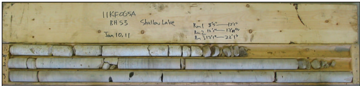
Photograph 1: Cores retrieved from borehole S3. Cores 5 to 7 from 2.6 to 6.7 m depth. RQD values ranged from 45 to 98%, indicating poor, fair to excellent rock quality.
