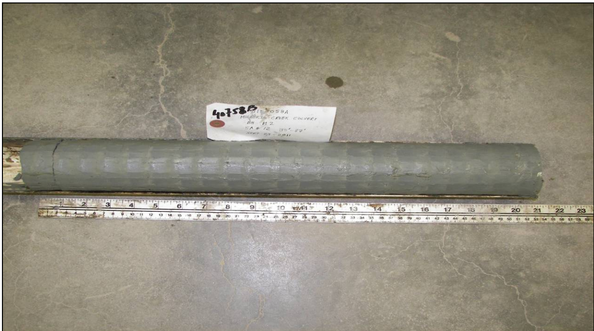
Photograph 2: Extruded thin wall sample from borehole M-2 at 10.7 to 11.3 m depth. Varved clay soils contain about 25 mm spacing less plastic clay soils (5 mm thick). (October 12, 2011)
