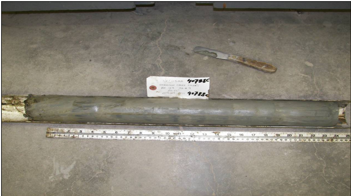
Photograph 1: Extruded thin wall sample from borehole M-3 at 6.1 to 6.7 m depth. Varved clay soils contain 50 mm spacing with high plastic layers (12 mm thick). (October 12, 2011)
