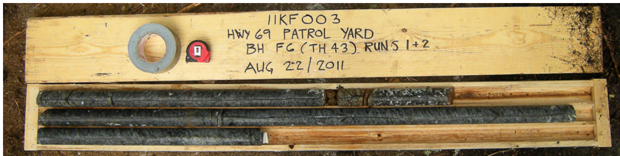
Photograph 2: Borehole F6, samples RC-1 and RC-2 from 0.4 to 3.6 m depth. The RQD values were 92 and 98%, indicating excellent quality bedrock.
