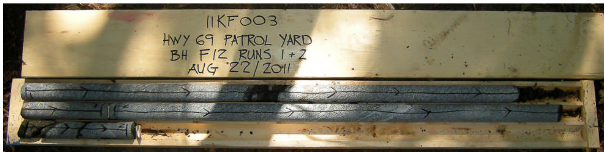
Photograph 4: Borehole F12, samples RC-1 and RC-2 from 0.0 to 3.1 m depth. The RQD values were 97 and 96%, indicating excellent quality bedrock.
