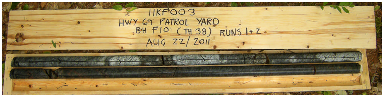
Photograph 3: Borehole F10, samples RC-1 and RC-2 from 0.0 to 3.1 m depth. The RQD values were 90 and 100%, indicating excellent quality bedrock.
