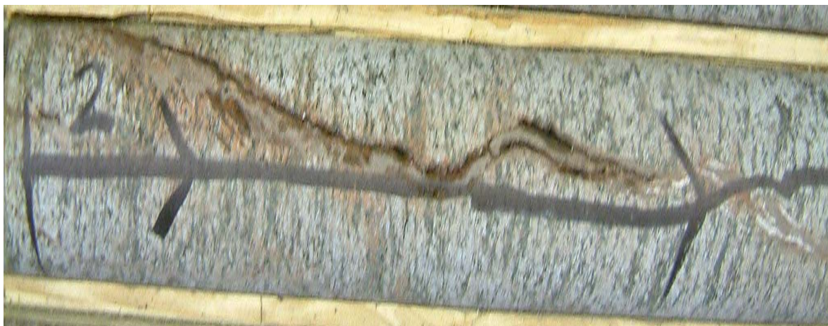
Core Photo 5: Borehole N2, Run 2, Close up view showing vertical partings upto 5 mm wide with secondary mineralization.
