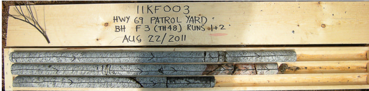
Photograph 1: Borehole F3, samples RC-1 and RC-2 from 0.0 to 3.3 m depth. The RQD values were 94 and 78%, indicating good to excellent quality bedrock.
