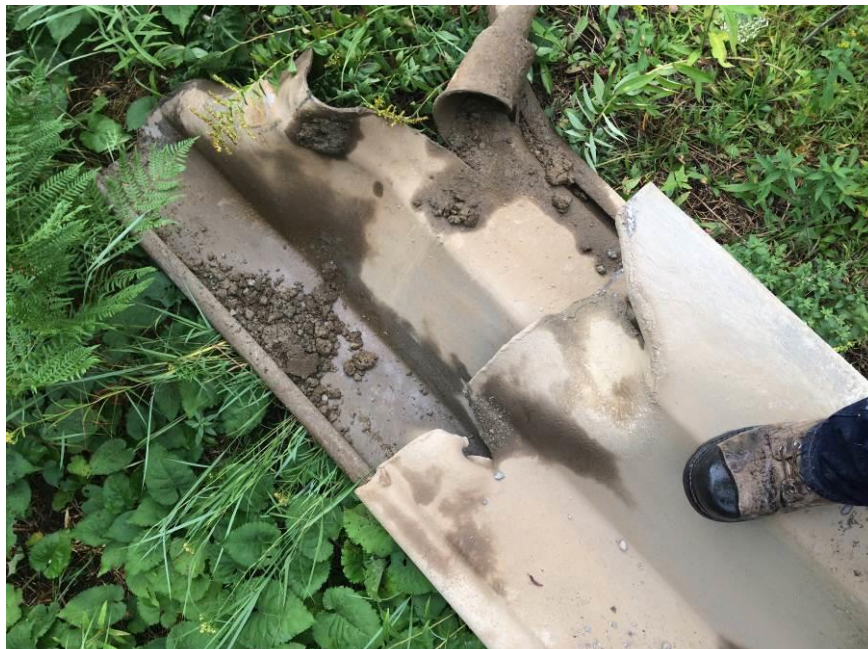
Toe of Test Pile No. 4 after Removal from Ground
