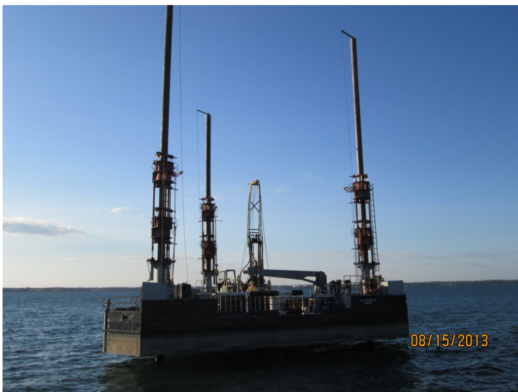
Jack-Up Barge at Borehole 13-06 (08/15/2013)
