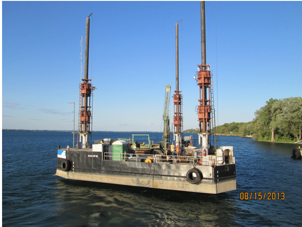
Jack-Up Barge at Borehole 13-06 (08/15/2013)
