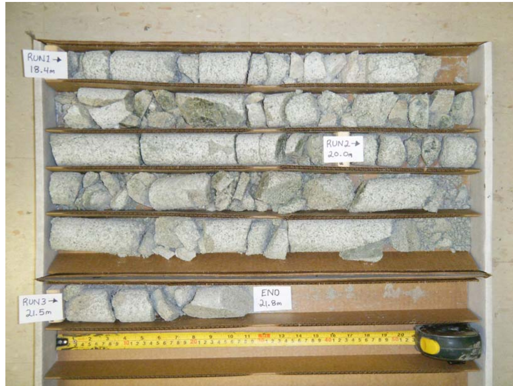
Bedrock Core Sample Borehole: MC-4 Runs: 1, 2 & 3 Depth: 18.4m – 21.8m
