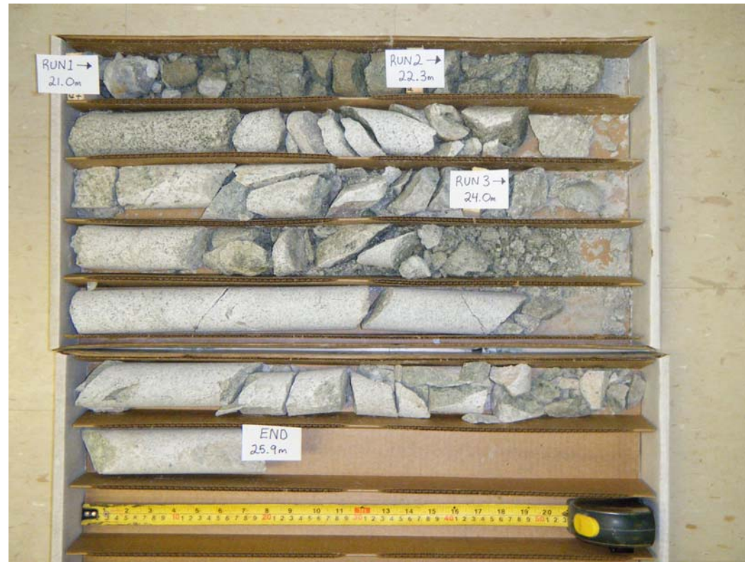
Bedrock Core Sample Borehole: MC-1 Runs: 1, 2 & 3 Depth: 21.0m – 25.9m
