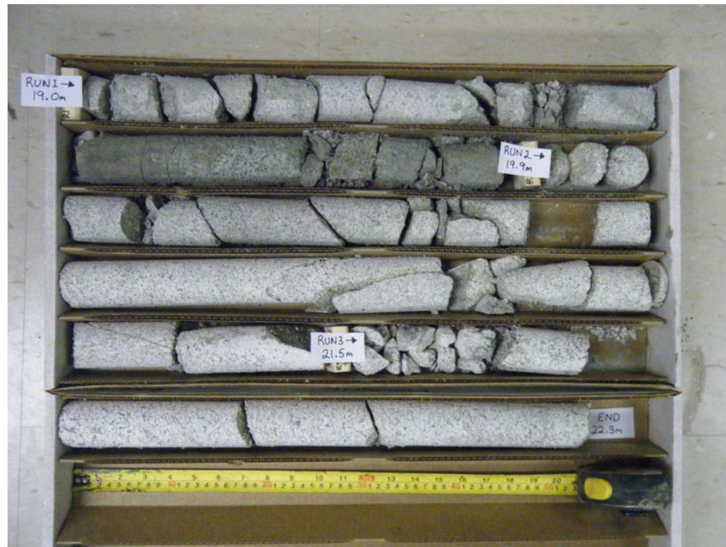
Bedrock Core Sample Borehole: MC-3 Runs: 1, 2 & 3 Depth: 19.0m – 22.3m
