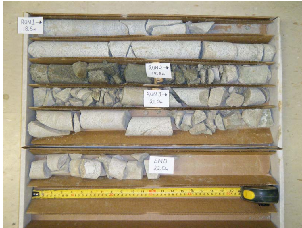
Bedrock Core Sample Borehole: MC-2 Runs: 1, 2 & 3 Depth: 18.5m – 22.0m
