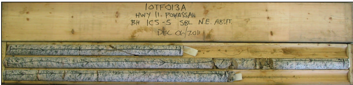
Photograph 2: Cores retrieved from borehole ICS-5. Cores 10 to 12 from 6.8 to 10.1 m depth. RQD values ranged from 80 to 100%, indicating good to excellent rock quality.
