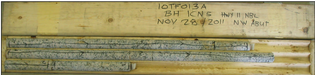
Photograph 2: Cores retrieved from borehole ICN-5. Cores 13 to 15 from 9.2 to 12.3 m depth. RQD values were 99 and 100%, indicating excellent rock quality.
