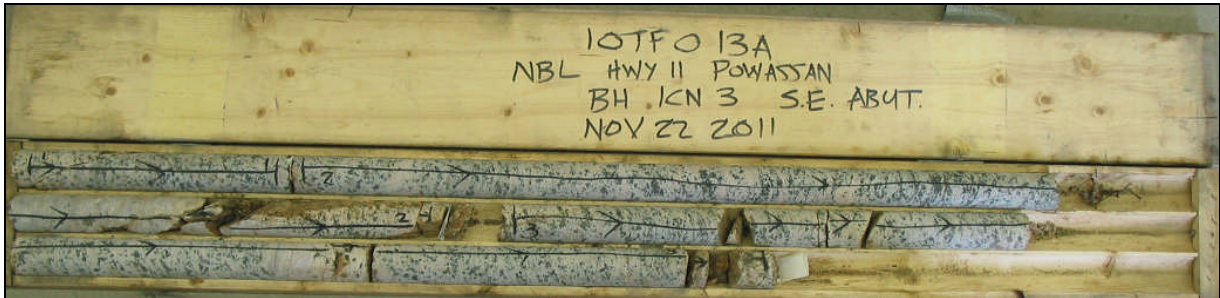
Photograph 1: Cores retrieved from borehole ICN-3. Cores 13 to 15 from 11.7 to 15.0 m depth. RQD values ranged from 75 to 82%, indicating good to excellent rock quality.
