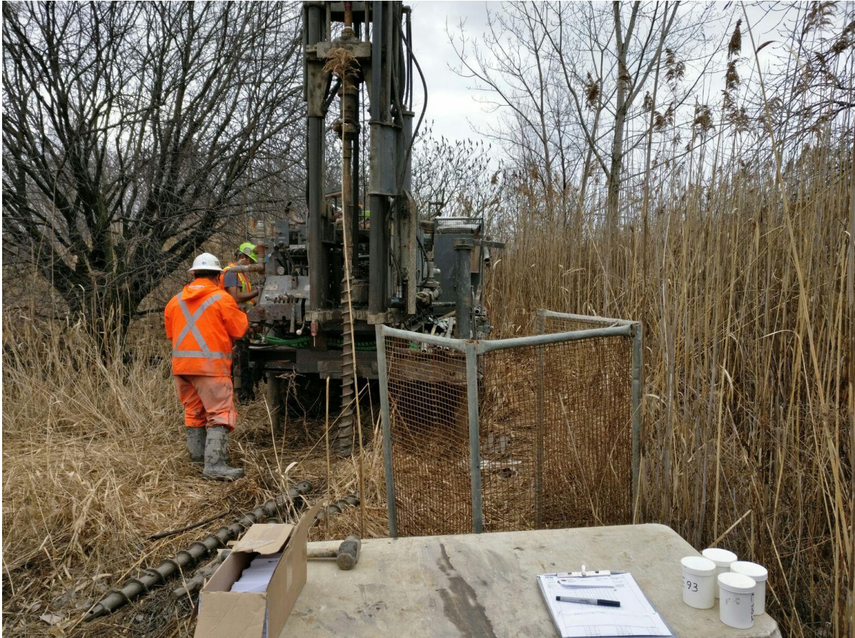
Photograph 4: Drilling for retaining wall RW2 (March 2, 2017).
