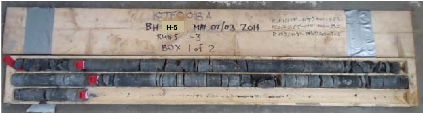
Photograph 1: Cores retrieved from borehole H-5. Rock cores 7 to 9 from 13.2 to 16.7 m depth. RQD values ranged from 44 to 88%, indicating poor becoming fair to good rock quality.
