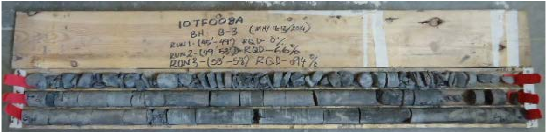
Photograph 1: Cores retrieved from borehole B-3. Rock Cores 12 to 14 from 13.7 to 17.7 m depth. RQD values ranged from 0 to 94%, indicating very poor becoming fair to excellent rock quality.
