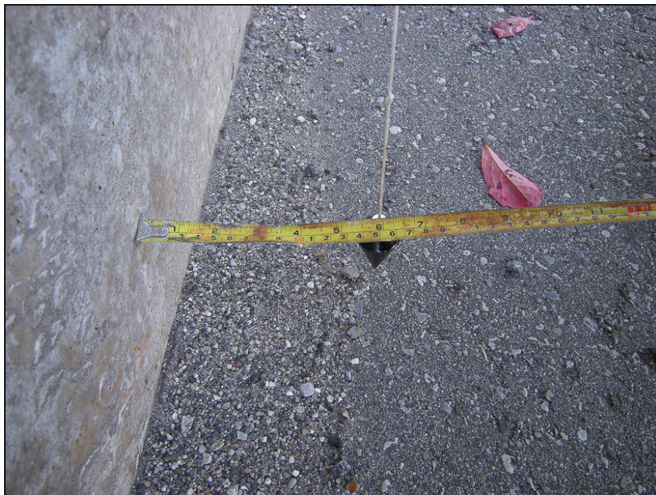
Photograph 8: Overhang measurement was taken from approximately 7 m north of south end of the retaining wall and it was approximately 152 mm (6 in.). (October 8, 2011).
