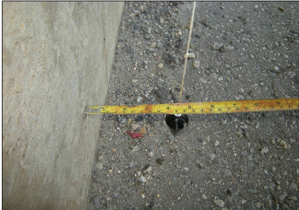
Photograph 9: Overhang measurement was taken from approximately (at double catch basin) 14 m north of south end of the retaining wall and it was approximately 114 mm (4.5 in.). (October 8, 2011)
