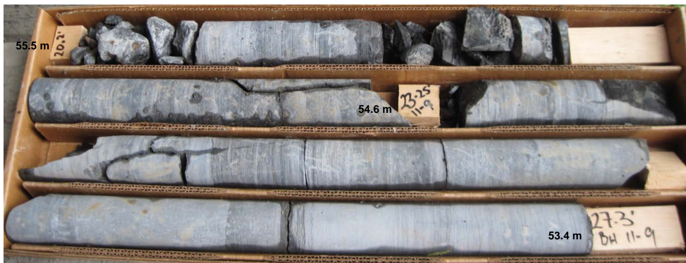
Photograph 9: BH 11-09: Rock Core Box 1: Elevation 55.5 to 53.4 metres.
