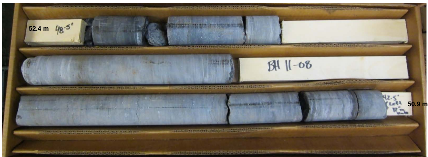
Photograph 8: BH 11-08 - Rock Core Box 2: Elevation 52.4 to 50.9 metres.
