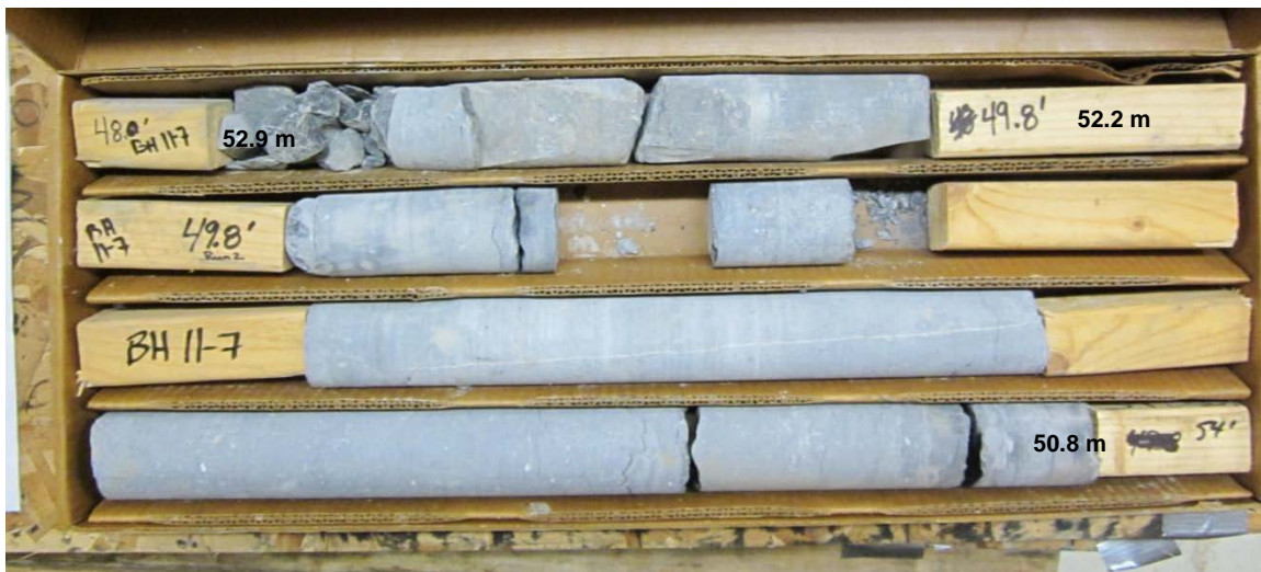
Photograph 5: BH 11-07 - Rock Core Box 1: Elevation 52.9 to 50.8 metres.
