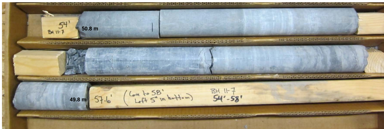
Photograph 6: BH 11-07 - Rock Core Box 2: Elevation 50.5 to 49.8 metres.
