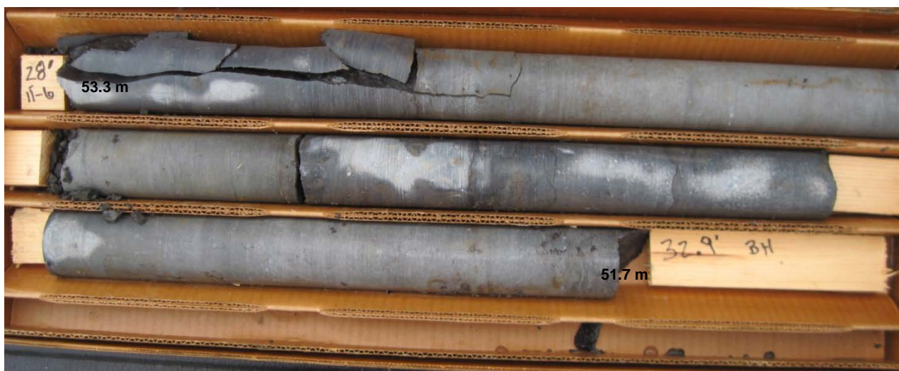
Photograph 4: BH 11-06 - Rock Core Box 2: Elevation 53.3 to 51.7 metres.
