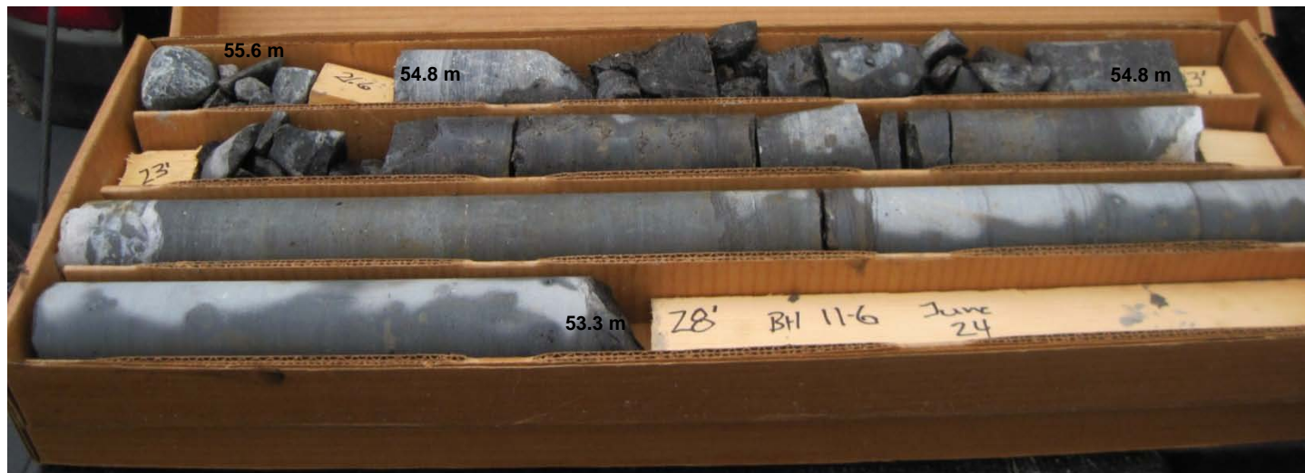
Photograph 3: BH 11-06 - Rock Core Box 1: Elevation 55.6 to 53.3 metres.
