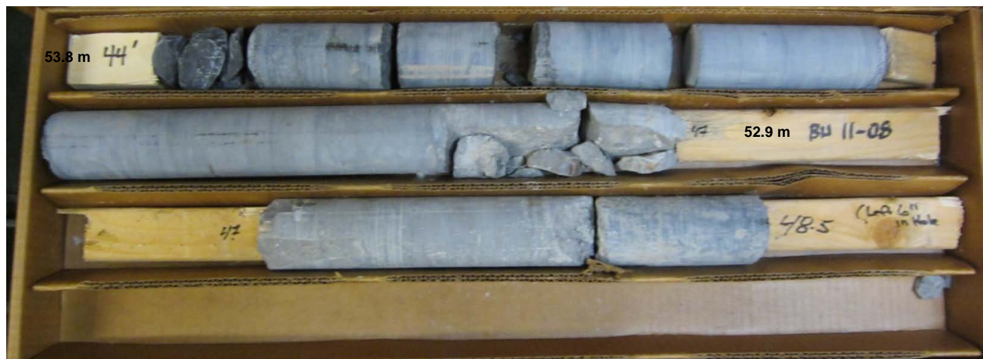
Photograph 7: BH 11-08 - Rock Core Box 1: Elevation 53.8 to 52.4 metres.
