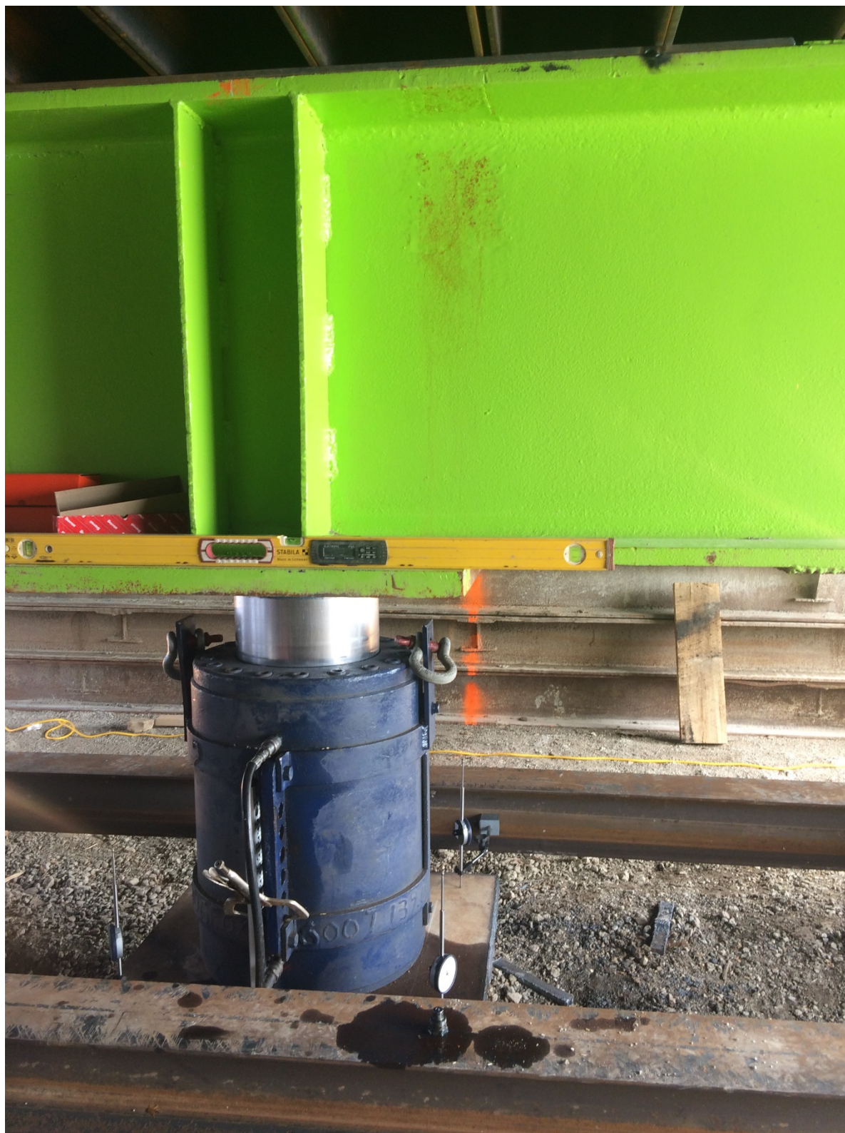
Photograph 6: Static load testing underway (note installation of level to monitor stability of reaction support beam)
