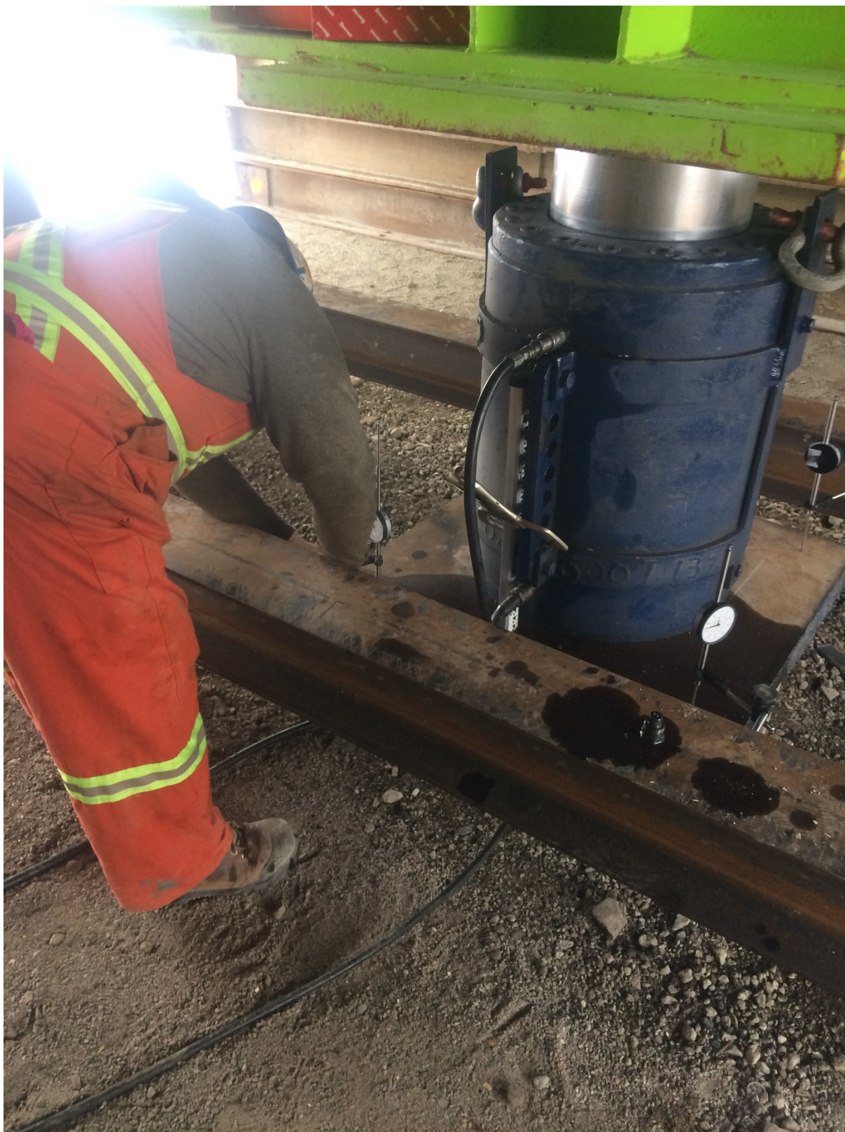
Photograph 5: Hydraulic jack and dial gauge set-up
