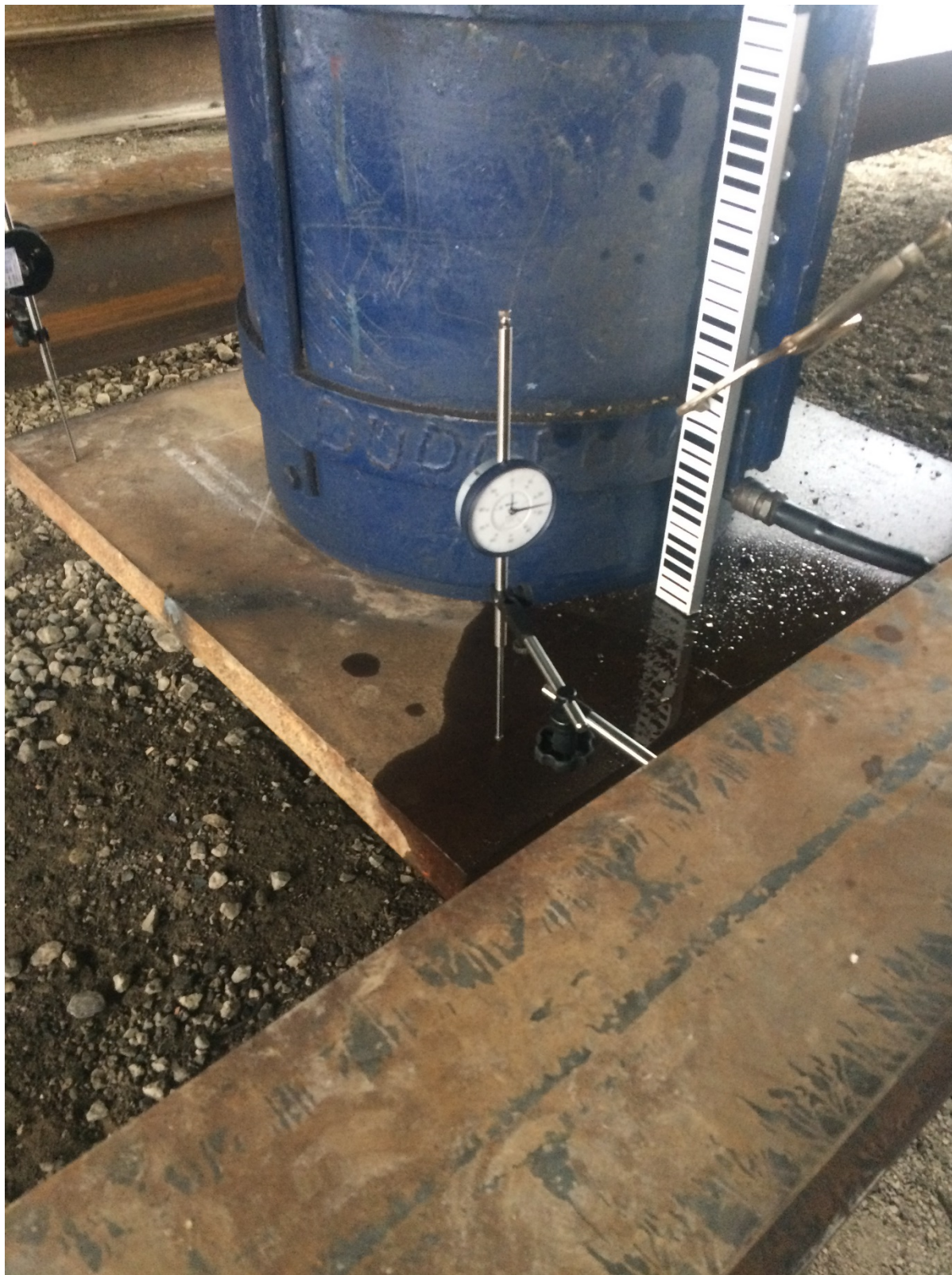
Photograph 3: Dial gauge(s) on independent reference beam
