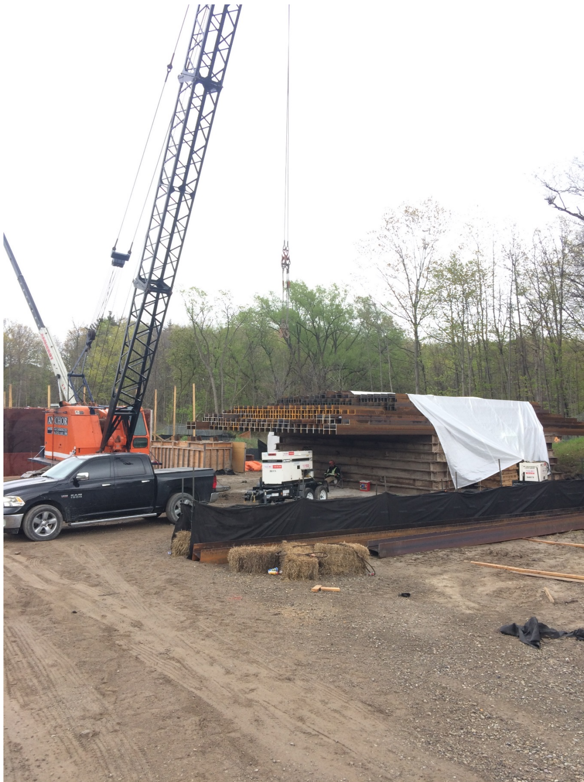
Photograph 2: Static pile load test reaction frame set-up (stacked H-piles)
