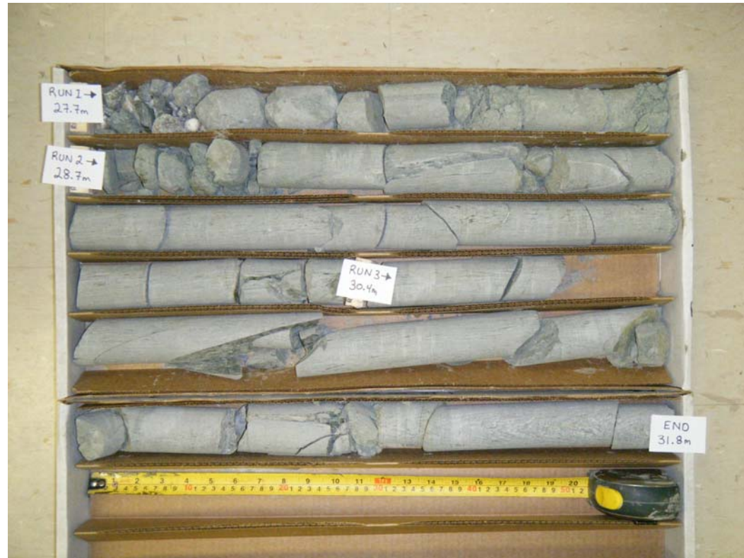
Bedrock Core Sample Borehole: C3 Runs: 1, 2 & 3 Depth: 27.7m – 31.8m
