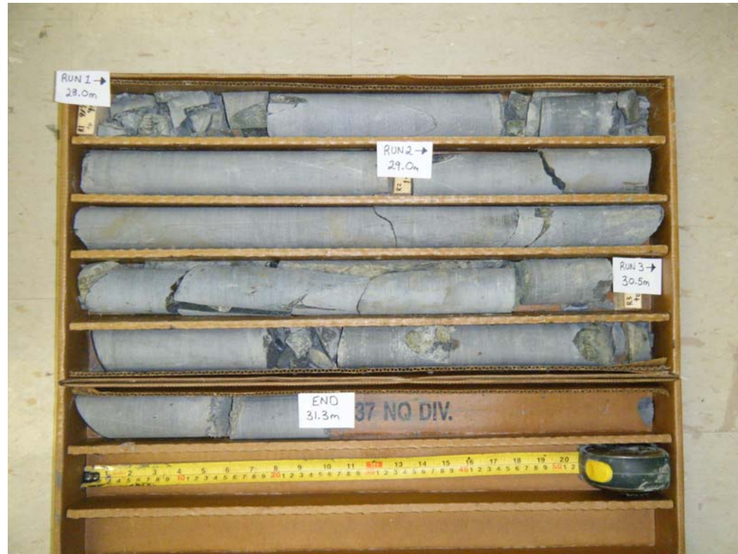
Bedrock Core Sample Borehole: C1 Runs: 1, 2 & 3 Depth: 28.0m – 31.3m
