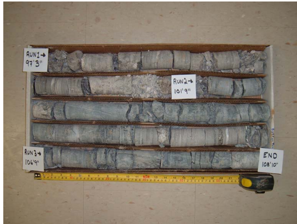
Bedrock Core Sample Borehole: TN3 Runs 1, 2 & 3 Depth: 29.6m – 33.2m
