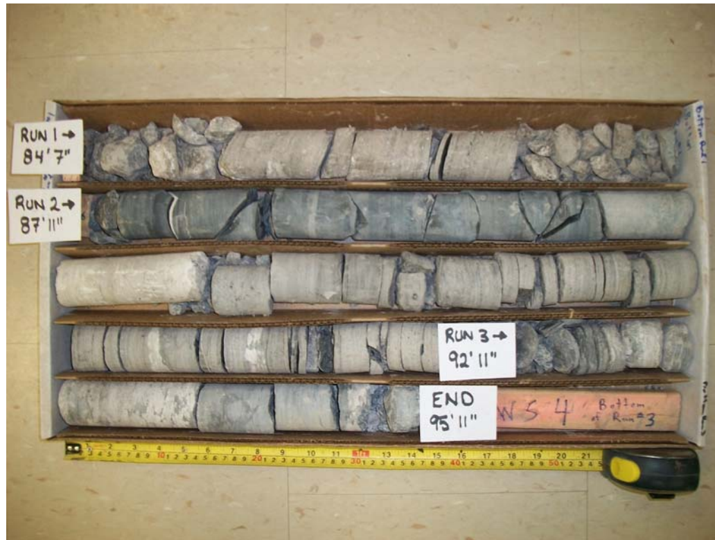
Bedrock Core Sample Borehole: WS4 Runs: 1, 2 & 3 Depth: 25.8m – 29.2m
