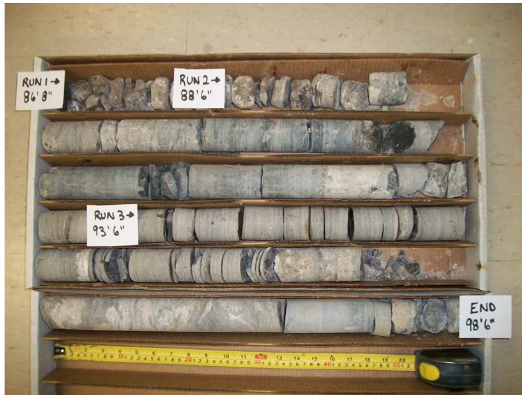
Bedrock Core Sample Borehole: WN3 Runs 1, 2 & 3 Depth: 26.4m – 30.0m
