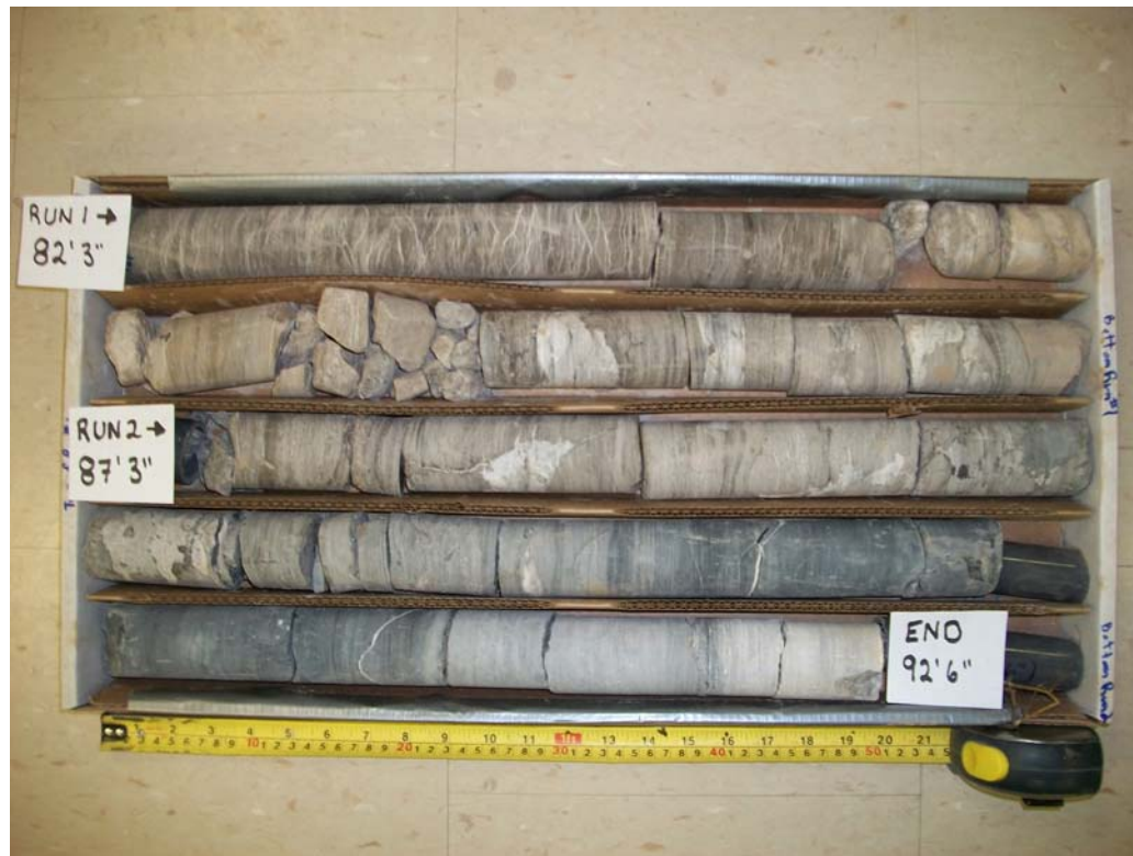
Bedrock Core Sample Borehole: WS3 Runs 1 & 2 Depth: 25.1m – 28.2m
