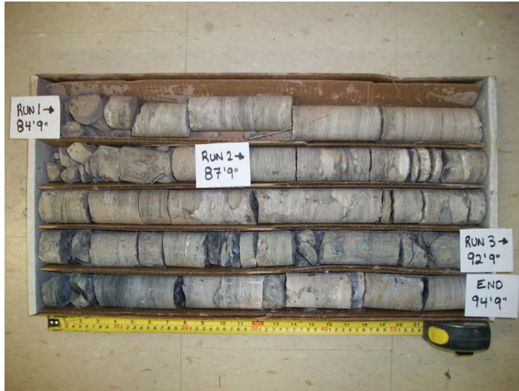
Bedrock Core Sample Borehole: WN4 Runs: 1, 2 & 3 Depth: 25.8m – 28.9m
