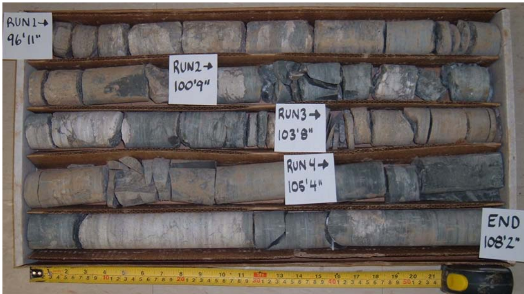
Bedrock Core Sample Borehole: TSEW4 Runs: 1, 2, 3 & 4 Depth: 29.5m – 33.0m
