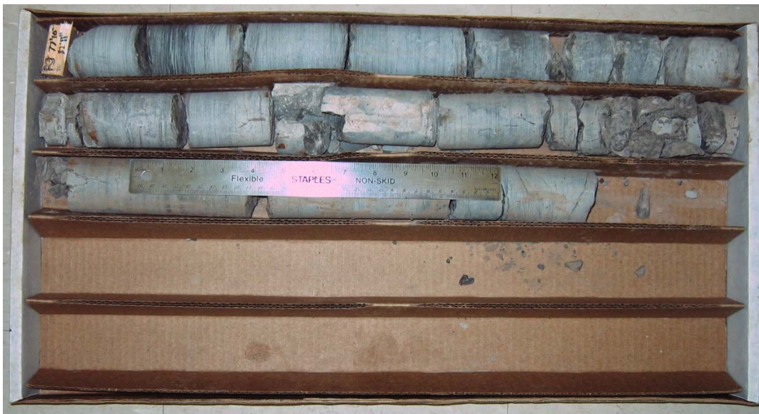
Bedrock Core Sample Borehole: W5 Runs: 1, 2 & 3 Depth: 21.3 m – 25.3 m
