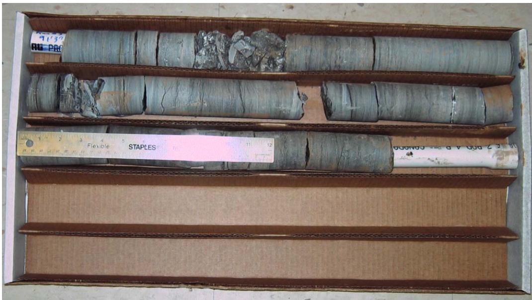
Bedrock Core Sample Borehole: W6 Runs: 1, 2 & 3 Depth: 25.1 m – 29.4 m
