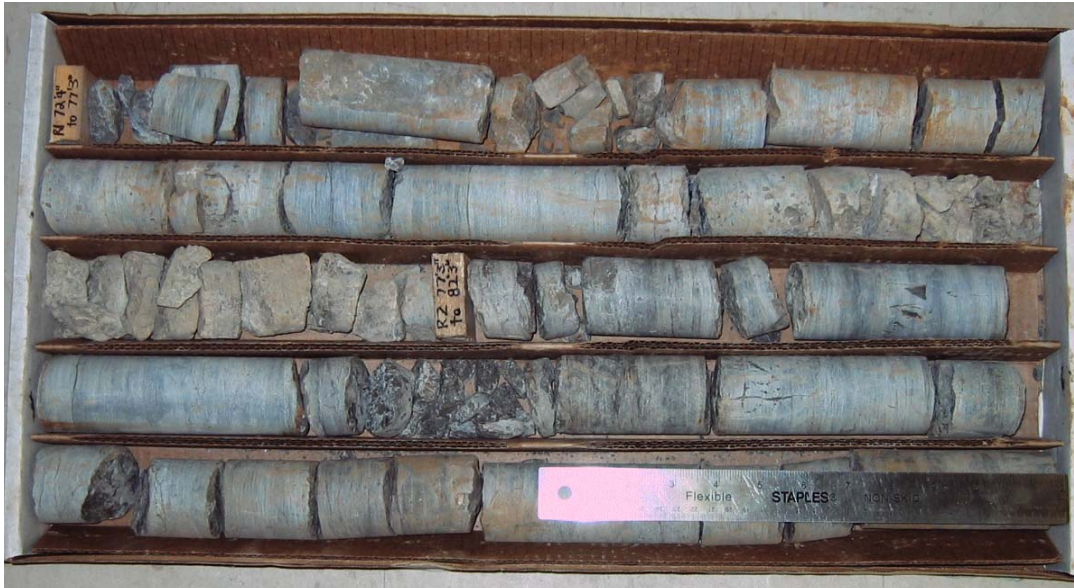
Bedrock Core Sample Borehole: W10 Runs: 1 & 2 Depth: 22.1 m – 25.1 m
