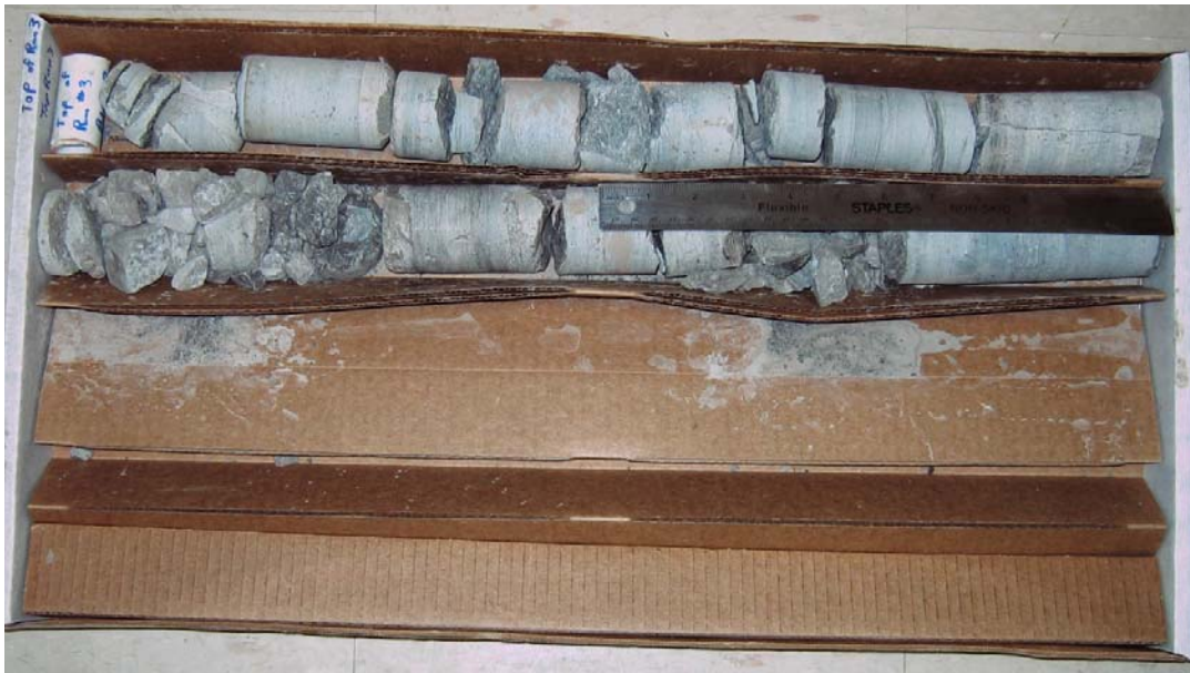
Bedrock Core Sample Borehole: W3 Runs: 1, 2 & 3 Depth: 26.8 m – 30.9 m
