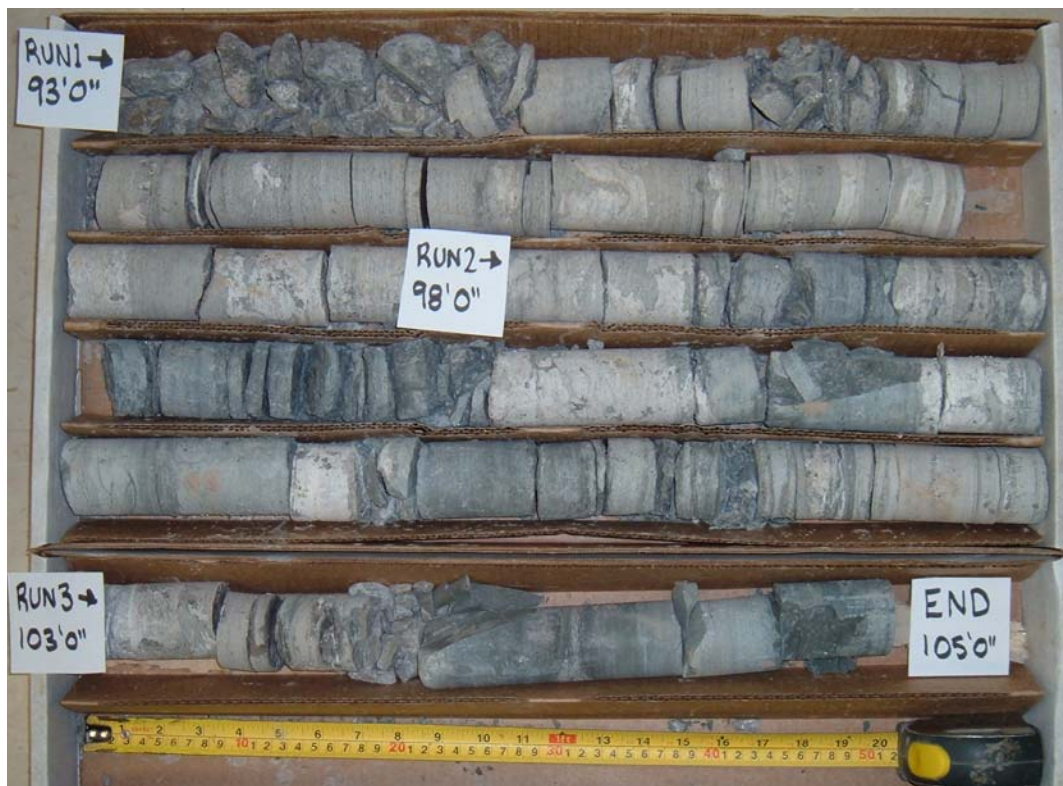
Bedrock Core Sample Borehole: TS4 Runs: 1, 2 & 3 Depth: 28.4m – 32.0m
