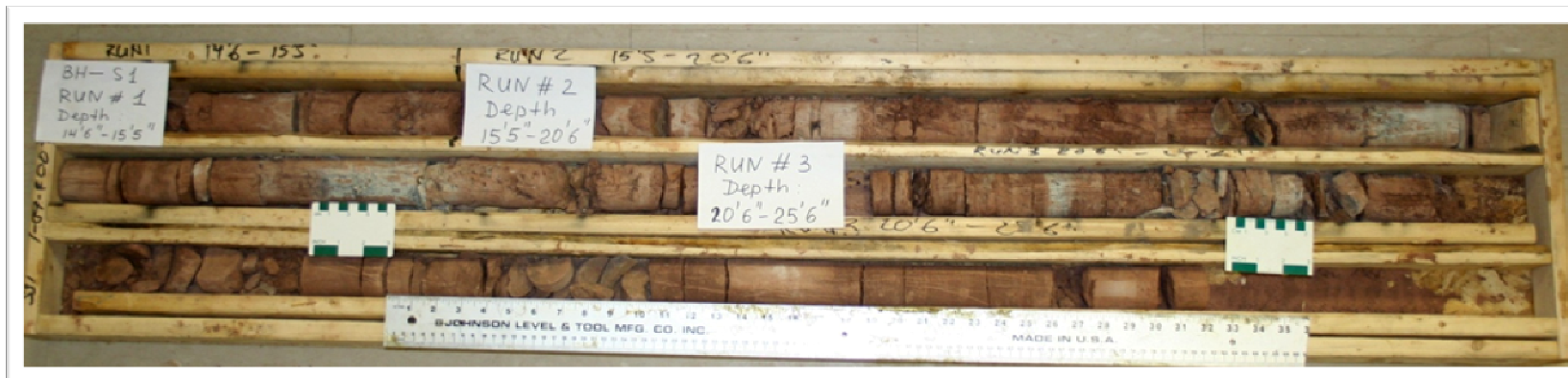
Bedrock Core Sample Borehole S1 Runs 1, 2 & 3 Depth 4.4m - 7.8m
