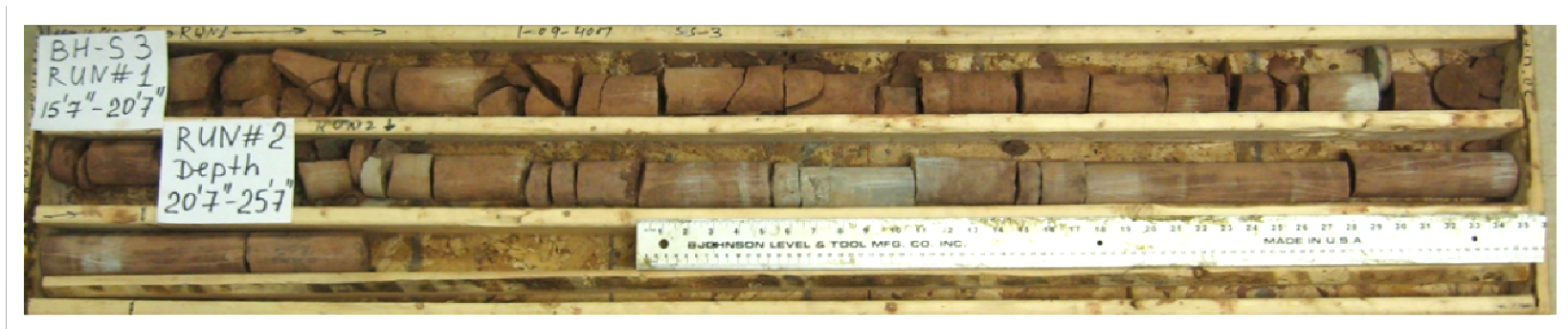
Bedrock Core Sample Borehole S3 Runs 1 & 2 Depth 4.8m - 7.8m
