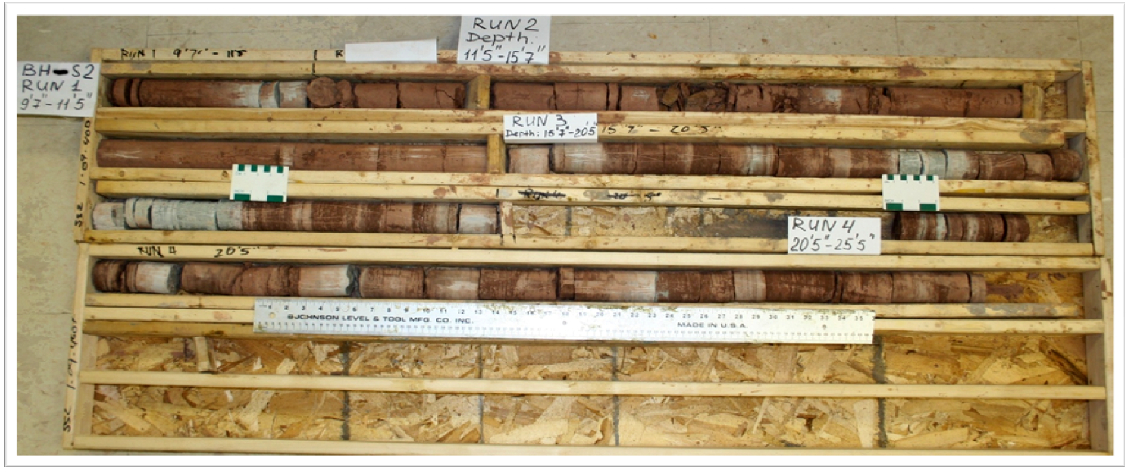
Bedrock Core Sample Borehole S2 Runs 1, 2, 3 & 4 Depth 2.9m - 7.8m
