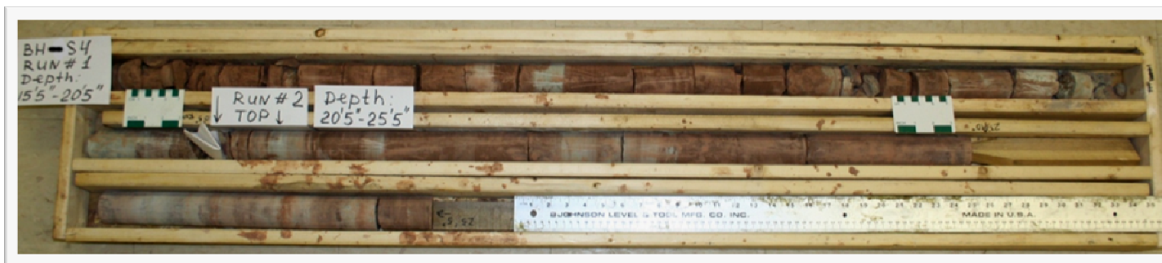
Bedrock Core Sample Borehole S4 Runs 1 & 2 Depth 4.7m - 7.8m
