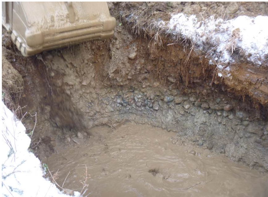
Testpit No. 2. Note: Cobbles encountered and groundwater in testpit.
