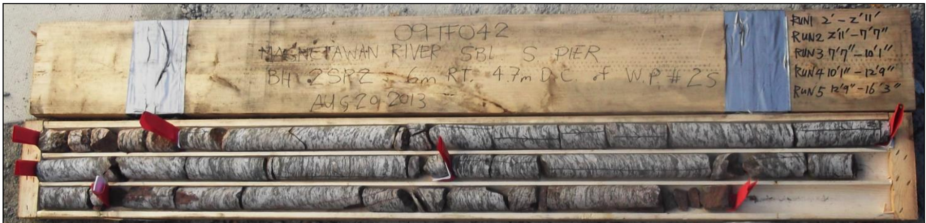
Photograph 2: Cores retrieved from borehole 2S-4. Rock cores 1 to 5 from 0.6 to 5.0 m depth. RQD values ranged from 0 to 92%, indicating very poor becoming fair to excellent rock quality.
