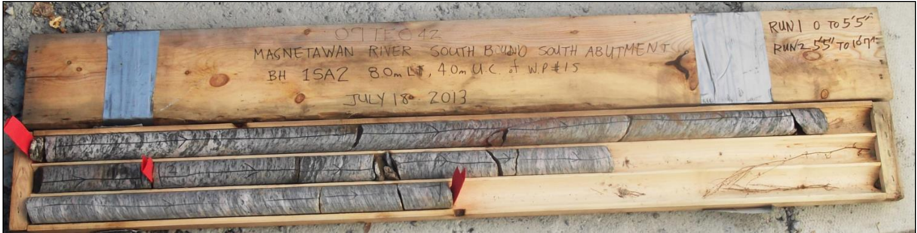
Photograph 1: Cores retrieved from borehole 1S-6. Rock cores 1 and 2 from 0.0 to 3.2 m depth. RQD values were 95 and 93%, indicating excellent rock quality.
