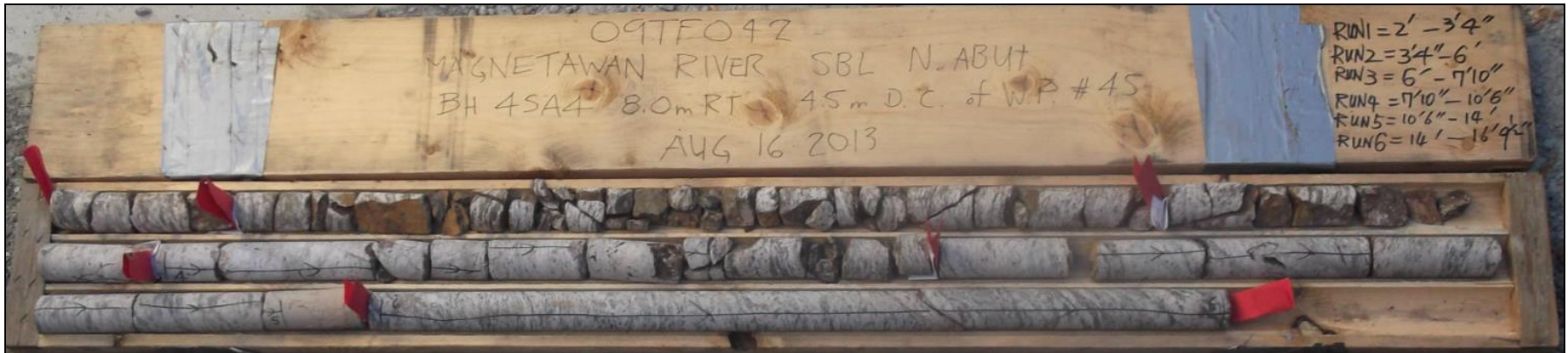
Photograph 3: Cores retrieved from borehole 4S-4. Rock cores 1 to 6 from 0.6 to 5.1 m depth. RQD values ranged from 0 to 100%, indicating very poor to poor becoming fair to excellent rock quality.
