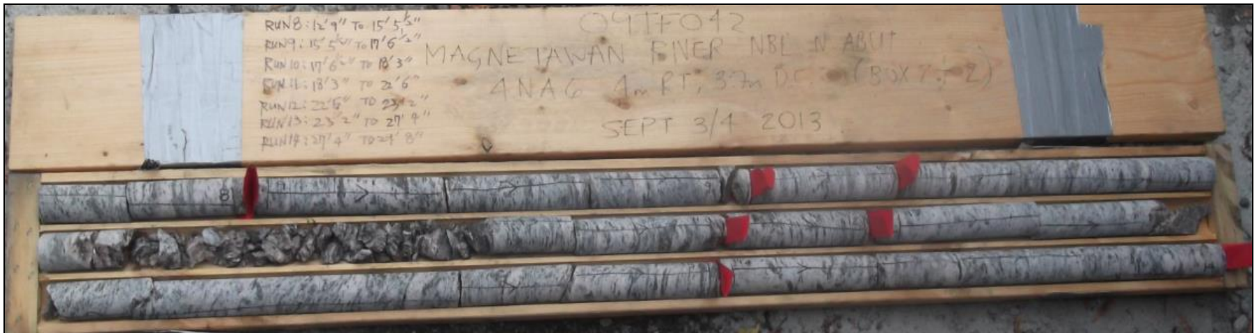
Photograph 4: Cores retrieved from borehole 4N-3 (box 2 of 2). Rock cores 8 to 14 from 4.5 to 9.0 m depth. RQD values ranged from 87 to 100%, indicating good to excellent rock quality.
