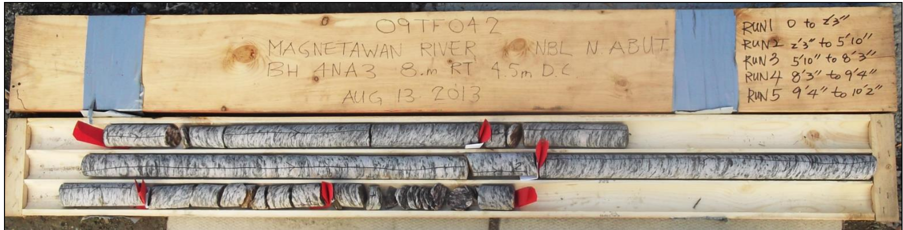
Photograph 5: Cores retrieved from borehole 4N-4. Rock cores 1 to 5 from 0.0 to 3.1 m depth. RQD values ranged from 53 to 98%, indicating excellent becoming fair to good rock quality.
