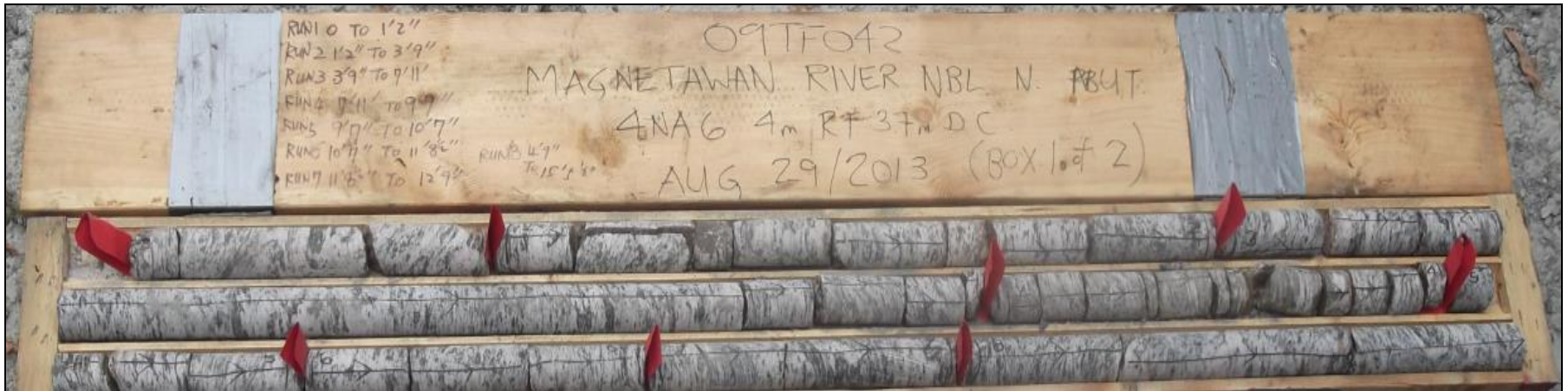
Photograph 3: Cores retrieved from borehole 4N-3 (box 1 of 2). Rock cores 1 to 8 from 0.0 to 4.5 m depth. RQD values ranged from 0 to 100%, indicating good to excellent locally very poor to fair rock quality.
