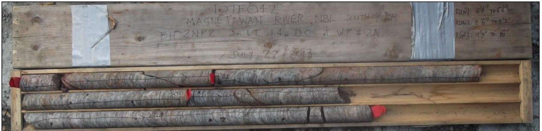
Photograph 2: Cores retrieved from borehole 2N-2. Rock cores 3 to 5 from 1.4 to 4.9 m depth. RQD values ranged from 87 to 100%, indicating good to excellent rock quality.
