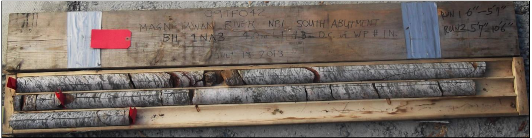
Photograph 1: Cores retrieved from borehole 1N-2. Rock cores 1 and 2 from 0.2 to 3.2 m depth. RQD values were 84 and 100%, indicating good to excellent rock quality.
