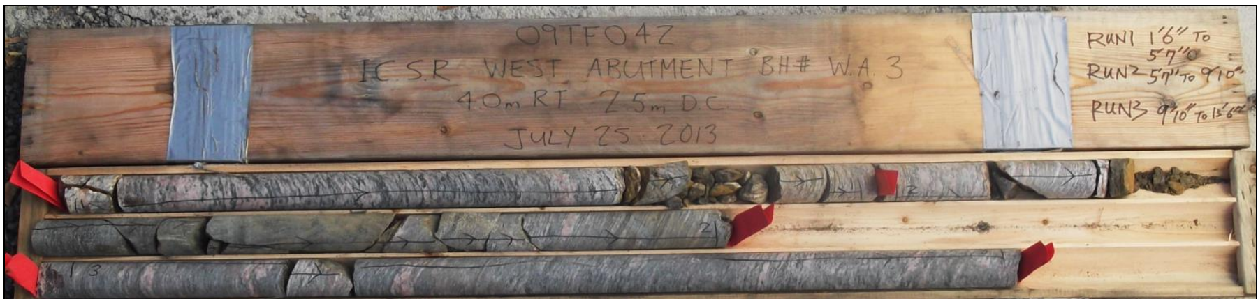
Photograph 2: Cores retrieved from borehole WA-3. Rock cores 2 to 4 from 0.4 to 4.1 m depth. RQD values ranged from 61 to 100%, indicating fair to excellent rock quality
