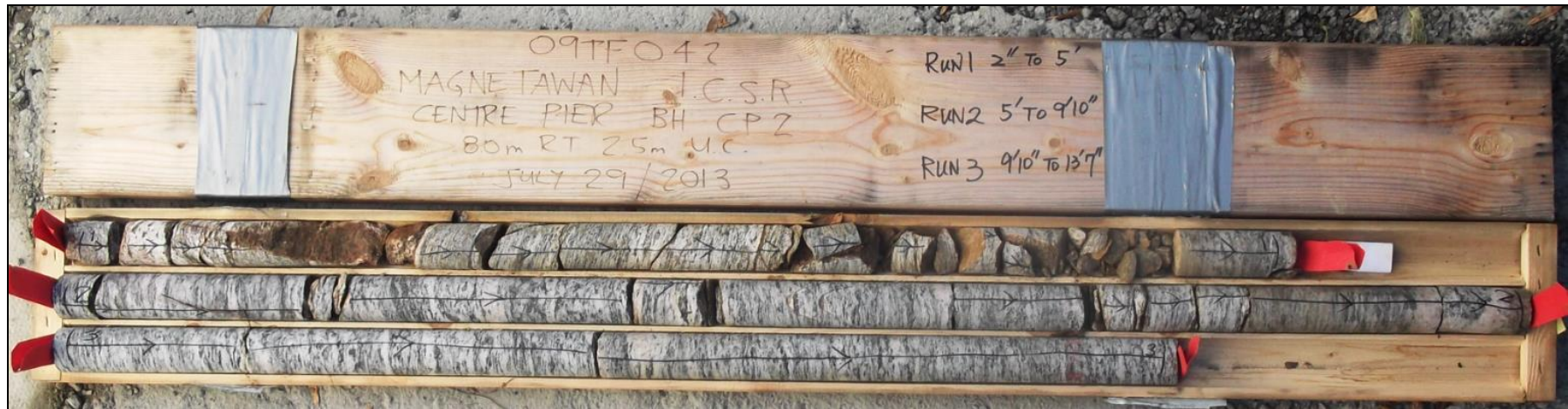
Photograph 6: Cores retrieved from borehole CP-9. Rock cores 1 to 3 from 0.1 to 4.1 m depth. RQD values ranged from 48 to 100%, indicating poor to excellent rock quality.
