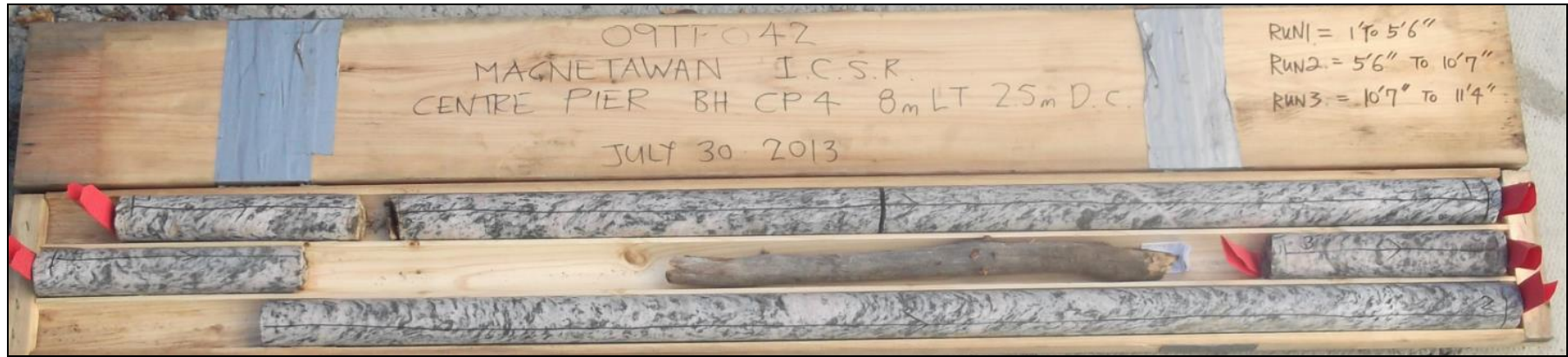
Photograph 5: Cores retrieved from borehole CP-1. Rock cores 1 to 3 from 0.3 to 3.5 m depth. RQD values ranged from 80 to 100%, indicating good to excellent rock quality.
