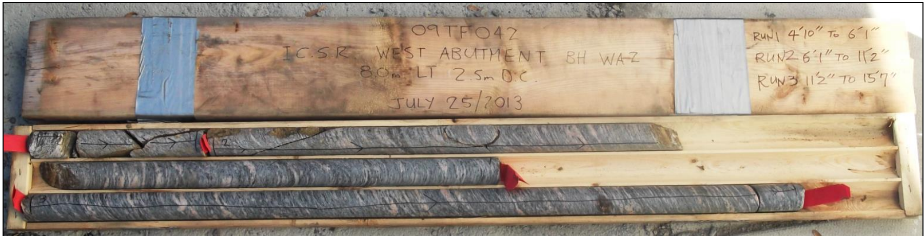
Photograph 1: Cores retrieved from borehole WA-1. Rock cores 3 to 5 from 1.5 to 4.7 m depth. RQD values ranged from 80 to 100%, indicating good to excellent rock quality.
