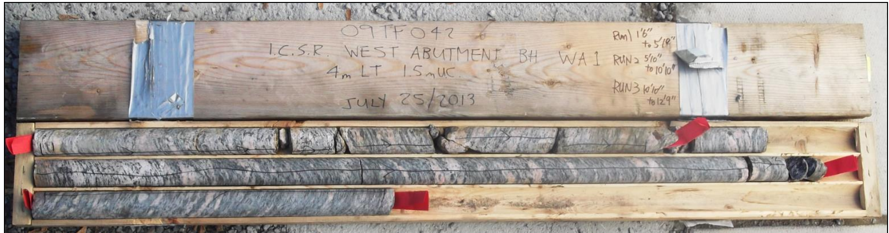
Photograph 3: Cores retrieved from borehole WA-7. Rock cores 2 to 4 from 0.4 to 3.9 m depth. RQD values ranged from 73 to 100%, indicating fair to excellent rock quality.
