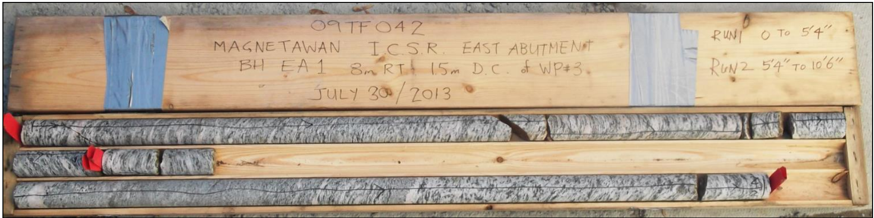
Photograph 7: Cores retrieved from borehole EA-4. Rock cores 1 and 2 from 0.0 to 3.2 m depth. RQD values were 93 and 97%, indicating excellent rock quality.
