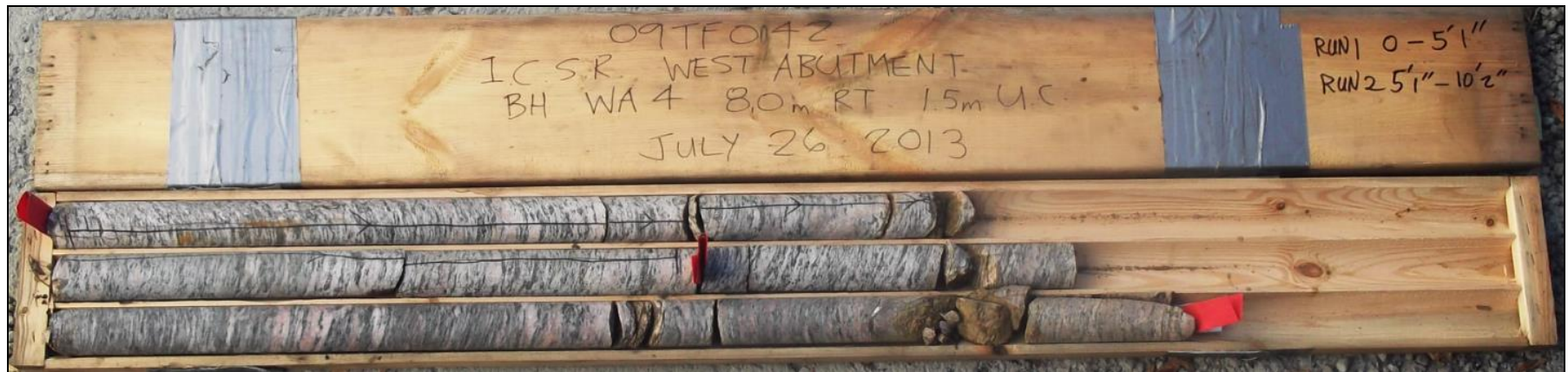
Photograph 4: Cores retrieved from borehole WA-9. Rock cores 1 and 2 from 0.0 to 3.1 m depth. RQD values were 98 and 79%, indicating excellent becoming good rock quality.
