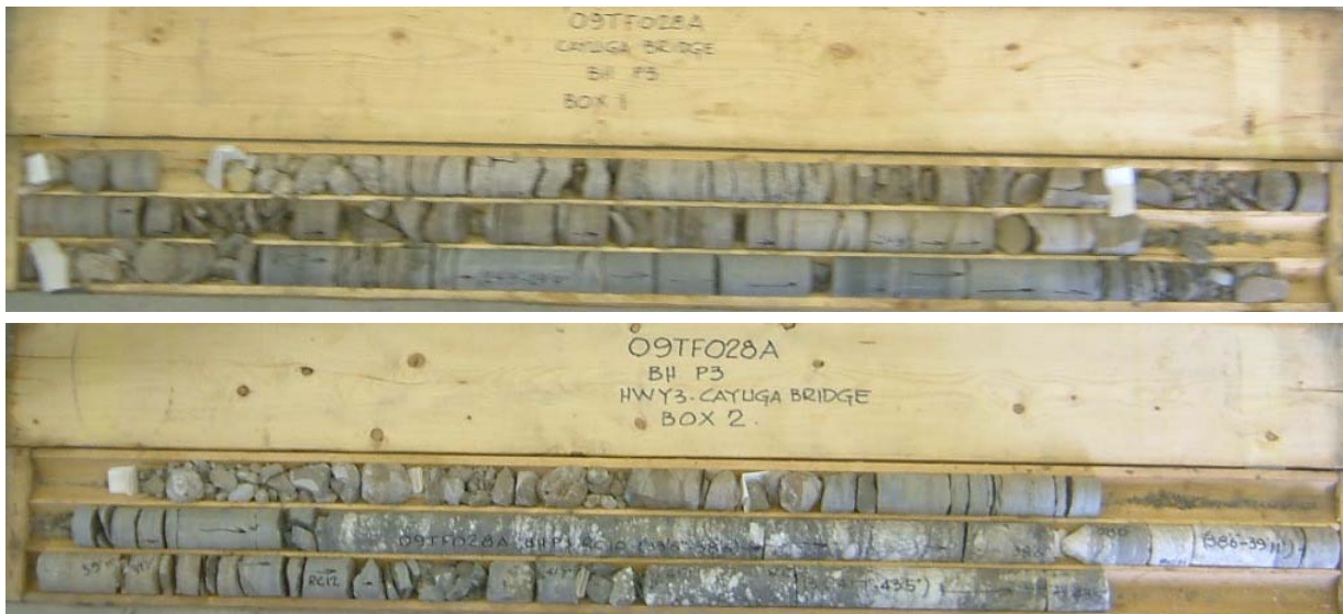
Photograph 9: Cores retrieved from borehole P3. Cores 5 to 13 from 4.9 to 12.9 m depth. RQD values ranged from 0 to 82%, indicating very poor becoming fair to good (locally very poor) rock quality.
