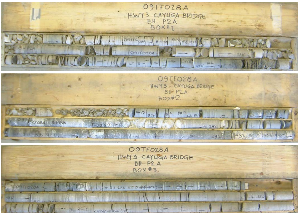
Photograph 8: Cores retrieved from borehole P2A. Cores 3 to 12 from 4.0 to 17.5 m depth. RQD values ranged from 0 to 73%, indicating very poor to poor becoming fair (locally poor) rock quality.
