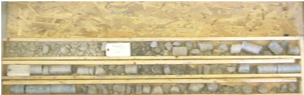
Photograph 13: Cores retrieved from borehole W2. Cores 12 to 16 from 10.1 to 16.8 m depth. RQD values ranged from 0 to 22%, indicating very poor rock quality.
