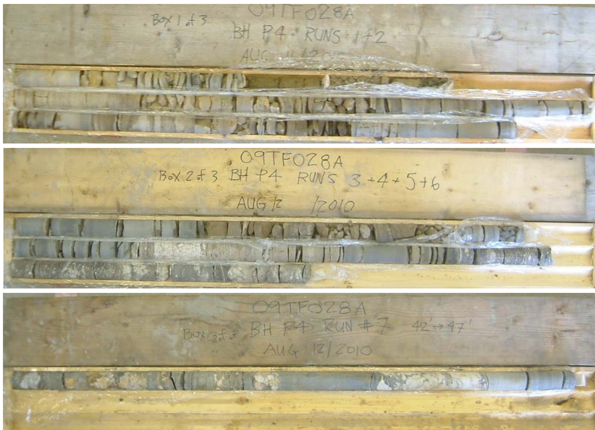
Photograph 11: Cores retrieved from borehole P4. Cores 6 to 12 from 4.6 to 14.3 m depth. RQD values ranged from 0 to 82%, indicating very poor to poor becoming good rock quality.
