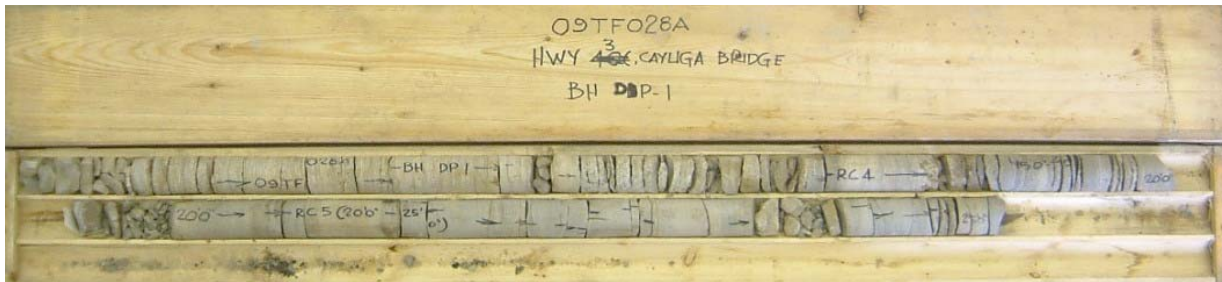
Photograph 1: Cores retrieved from borehole DP1. Cores 4 and 5 from 4.3 to 7.3 m depth. RQD value was 18% for both cores, indicating very poor rock quality.
