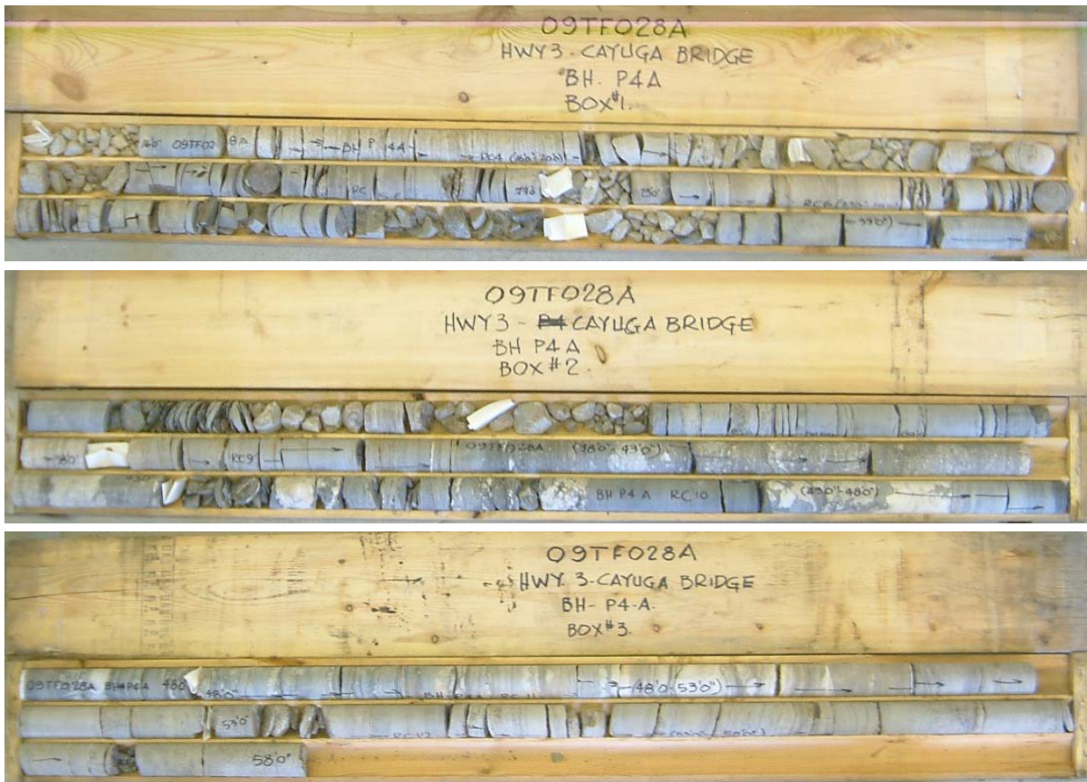
Photograph 12: Cores retrieved from borehole P4A. Cores 4 to 12 from 4.6 to 17.4 m depth. RQD values ranged from 0 to 74%, indicating very poor becoming poor to fair rock quality.
