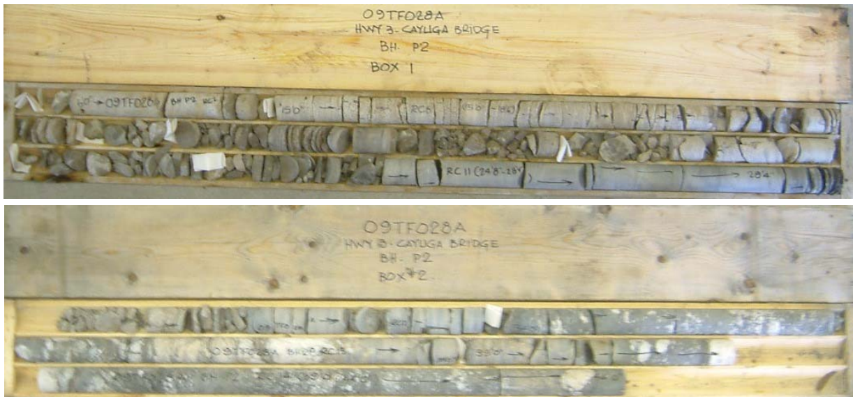
Photograph 7: Cores retrieved from borehole P2. Cores 6 to 14 from 4.3 to 13.1 m depth. RQD values ranged from 0 to 93%, indicating very poor to fair becoming good to excellent rock quality.
