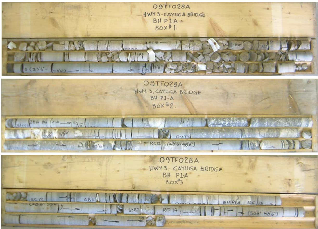
Photograph 6: Cores retrieved from borehole P1A. Cores 5 to 14 from 4.3 to 17.5 m depth. RQD values ranged from 0 to 83%, indicating very poor becoming fair to good rock quality.
