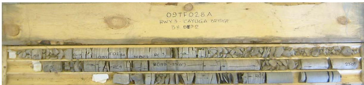
Photograph 2: Cores retrieved from borehole DP2. Cores 3 to 5 from 4.3 to 7.6 m depth. RQD values ranged from 0 to 40%, indicating very poor to poor rock quality.
