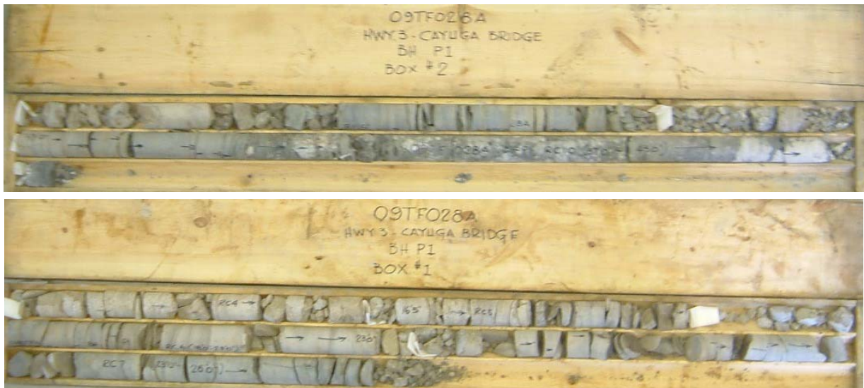
Photograph 5: Cores retrieved from borehole P1. Cores 4 to 10 from 3.8 to 12.8 m depth. RQD values ranged from 0 to 75%, indicating very poor becoming good rock quality.
