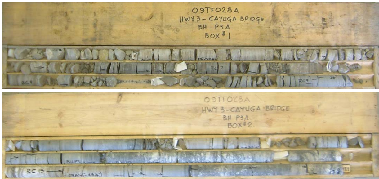
Photograph 10: Cores retrieved from borehole P3A. Cores 5 to 16 from 4.3 to 17.4 m depth. RQD values ranged from 0 to 91%, indicating very poor becoming poor to fair (locally excellent) rock quality.
