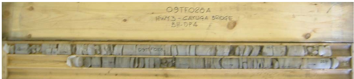
Photograph 4: Cores retrieved from borehole DP4. Cores 4 and 5 from 4.4 to 7.3 m depth. RQD values were 0 and 8% respectively, indicating very poor rock quality.
