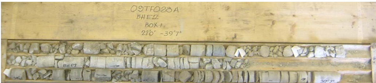
Photograph 14: Cores retrieved from borehole E1. Cores 10 to 14 from 8.7 to 13.9 m depth. RQD values ranged from 0 to 23%, indicating very poor rock quality.
