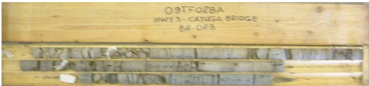
Photograph 3: Cores retrieved from borehole DP3. Cores 4 to 7 from 4.6 to 8.2 m depth. RQD values ranged from 0 to 33%, indicating very poor to poor rock quality.
