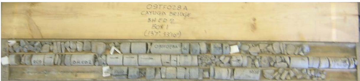
Photograph 15: Cores retrieved from borehole E2. Cores 9 to 13 from 6.7 to 13.4 m depth. RQD values ranged from 0 to 51%, indicating very poor becoming fair rock quality.
