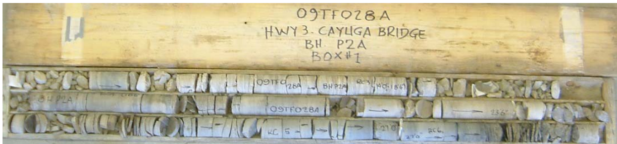
Photograph 7: Cores retrieved from borehole P2. Cores 6 to 14 from 4.3 to 13.1 m depth. RQD values ranged from 0 to 93%, indicating very poor to fair becoming good to excellent rock quality.
