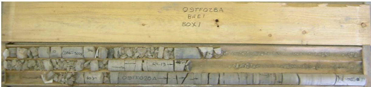
Photograph 14: Cores retrieved from borehole E1. Cores 10 to 14 from 8.7 to 13.9 m depth. RQD values ranged from 0 to 23%, indicating very poor rock quality.
