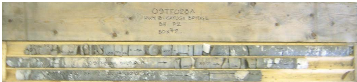
Photograph 7: Cores retrieved from borehole P2. Cores 6 to 14 from 4.3 to 13.1 m depth. RQD values ranged from 0 to 93%, indicating very poor to fair becoming good to excellent rock quality.
