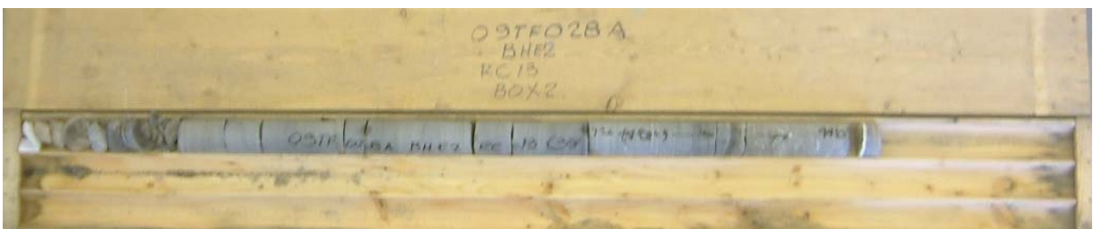
Photograph 15: Cores retrieved from borehole E2. Cores 9 to 13 from 6.7 to 13.4 m depth. RQD values ranged from 0 to 51%, indicating very poor becoming fair rock quality.
