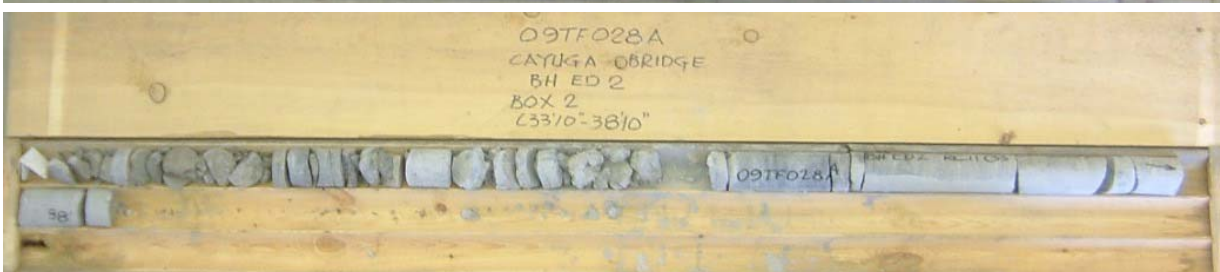
Photograph 16: Cores retrieved from borehole DE2. Cores 6 to 11 from 4.1 to 11.8 m depth. RQD values ranged from 0 to 29%, indicating very poor to poor rock quality.
