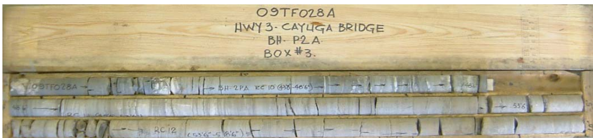
Photograph 8: Cores retrieved from borehole P2A. Cores 3 to 12 from 4.0 to 17.5 m depth. RQD values ranged from 0 to 73%, indicating very poor to poor becoming fair (locally poor) rock quality.
