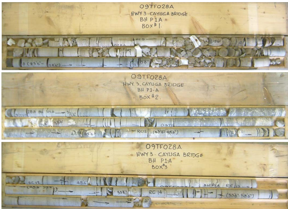
Photograph 6: Cores retrieved from borehole P1A. Cores 5 to 14 from 4.3 to 17.5 m depth. RQD values ranged from 0 to 83%, indicating very poor becoming fair to good rock quality.
