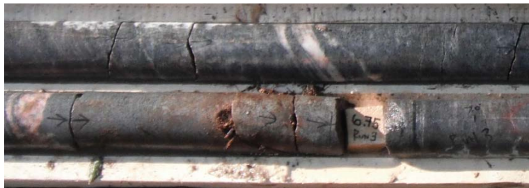
50 mm thick infilling of rootlets/organic matter at 2.0 m depth
