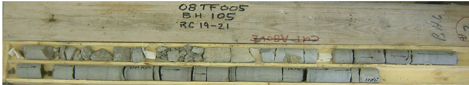
Photograph 1: Rock core from borehole 105. Samples RC19 to RC21 taken from 36.2 to 38.9 m depths.
