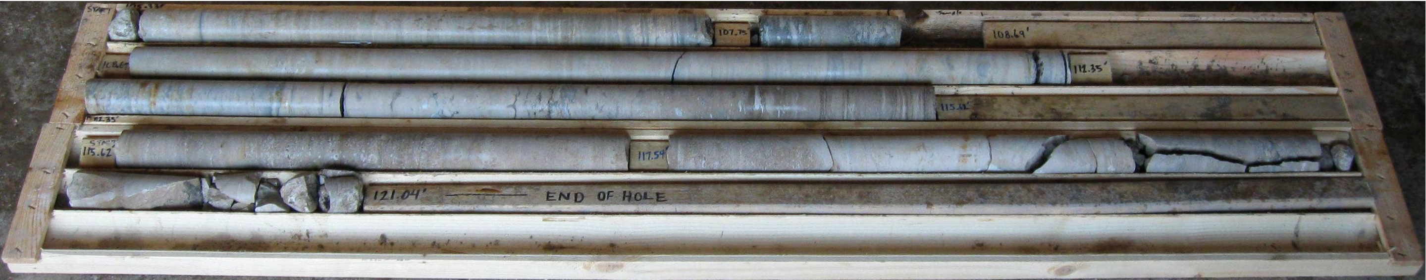
Photo 12: Borehole No. 119 – Rock Core. Elevation 150.40 metres to 145.54 metres.
