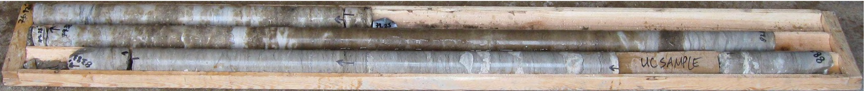
Photo 32: Borehole No. 166 – Rock Core. Elevation 155.73 metres to 152.08 metres.
