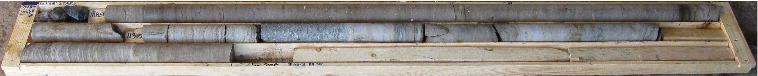
Photo 14: Borehole No. 127 – Rock Core. Elevation 148.47 metres to 145.16 metres.
