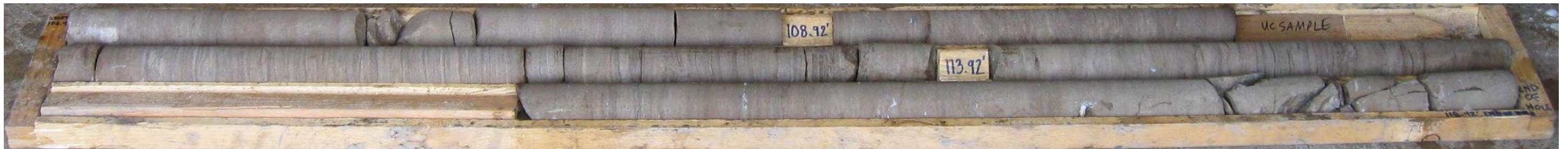
Photo 22: Borehole No. 141 – Rock Core. Elevation 149.33 metres to 145.47 metres.
