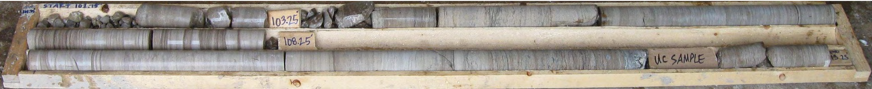
Photo 25: Borehole No. 149 – Rock Core. Elevation 149.97 metres to 146.46 metres.
