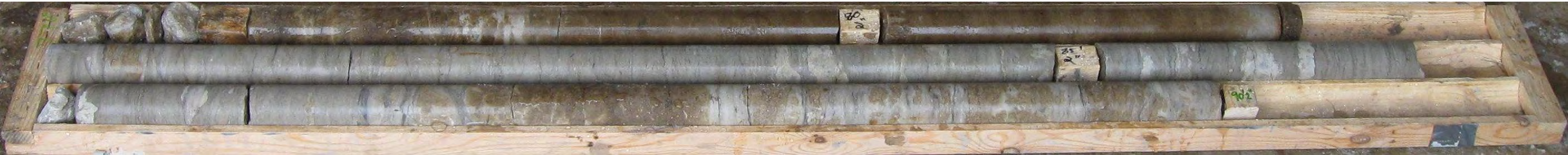
Photo 31: Borehole No. 164 – Rock Core. Elevation 155.59 metres to 151.58 metres.
