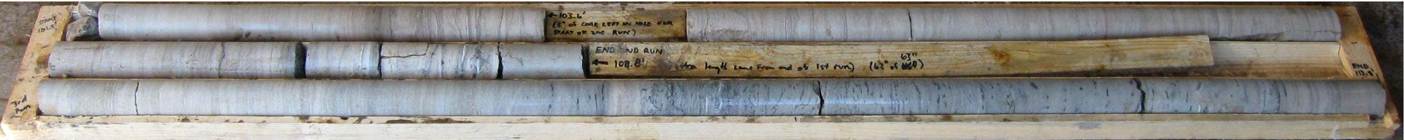
Photo 3: Borehole No. 104 – Rock Core. Elevation 155.70 metres to 151.45 metres.
