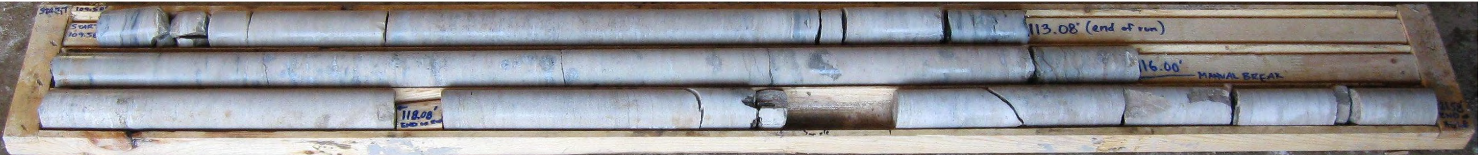
Photo 1: Borehole No. 101 – Rock Core. Elevation 154.05 metres to 150.31 metres.
