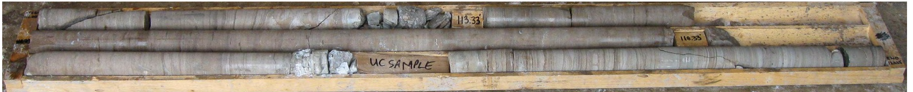
Photo 21: Borehole No. 140 – Rock Core. Elevation 148.88 metres to 144.41 metres.
