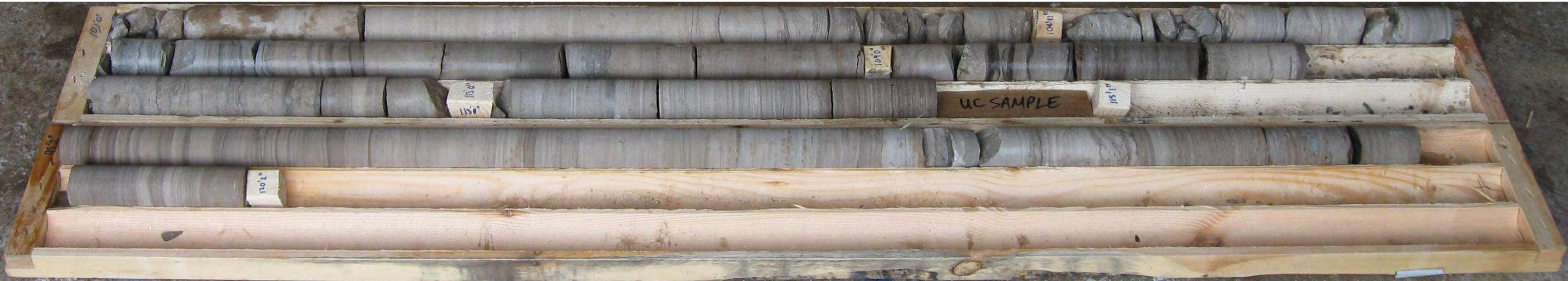
Photo 26: Borehole No. 152 – Rock Core. Elevation 149.37 metres to 143.53 metres.
