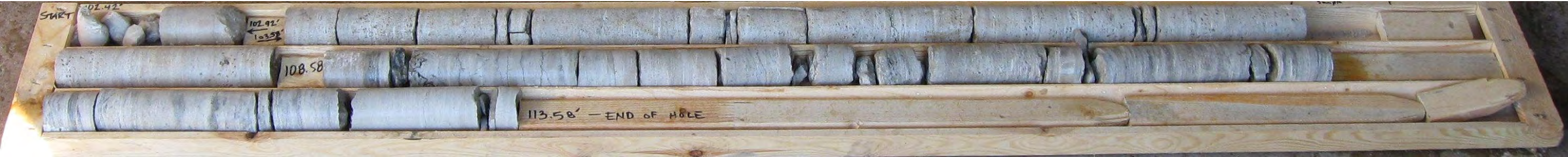
Photo 4: Borehole No. 105 – Rock Core. Elevation 155.68 metres to 151.54 metres.
