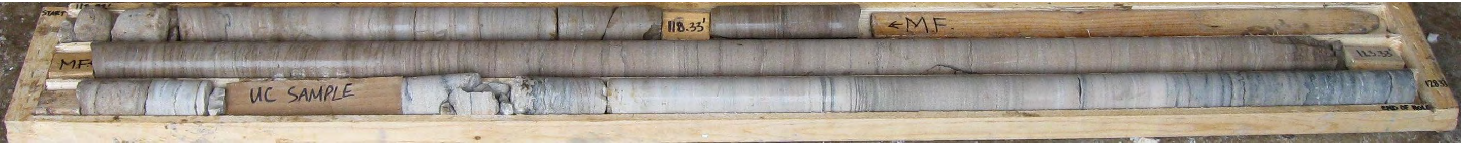
Photo 20: Borehole No. 139 – Rock Core. Elevation 147.04 metres to 143.19 metres.
