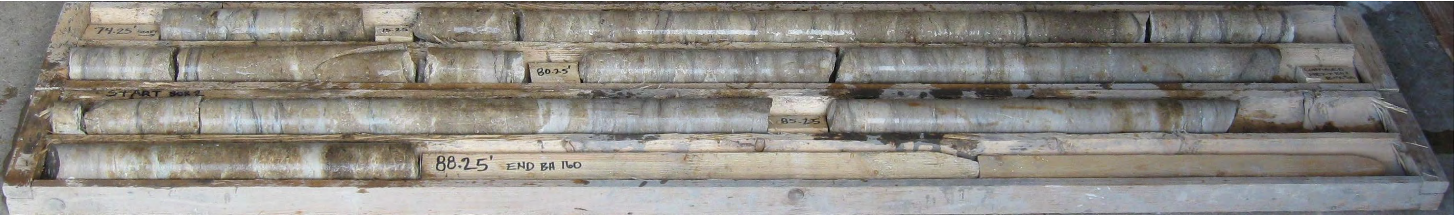
Photo 29: Borehole No. 160 – Rock Core. Elevation 156.26 metres to 151.62 metres.
