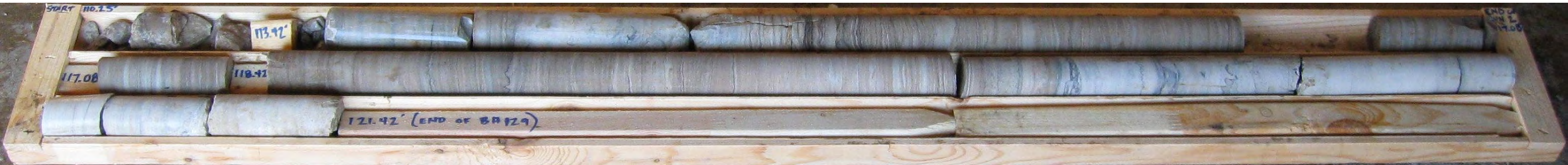
Photo 15: Borehole No. 129 – Rock Core. Elevation 147.88 metres to 143.78 metres.
