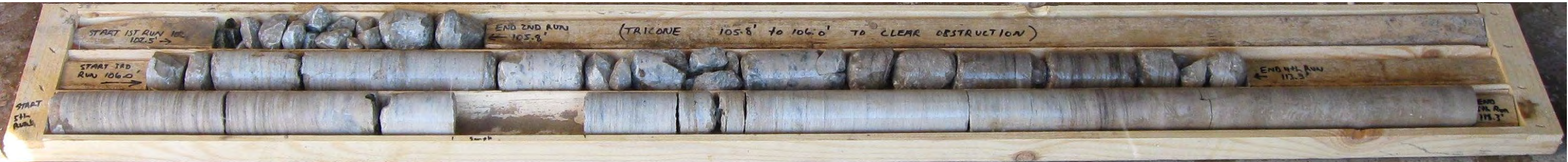
Photo 8: Borehole No. 113 – Rock Core. Elevation 153.01 metres to 148.35 metres.
