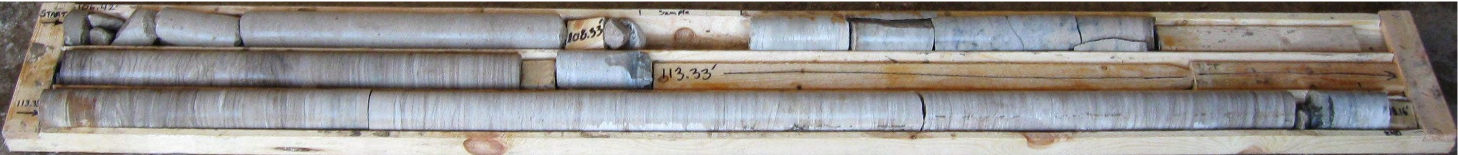
Photo 10: Borehole No. 116 – Rock Core. Elevation 151.66 metres to 147.58 metres.
