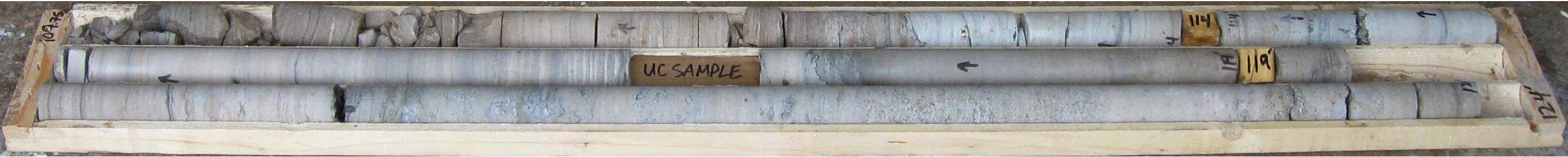
Photo 17: Borehole No. 132 – Rock Core. Elevation 148.04 metres to 143.67 metres.
