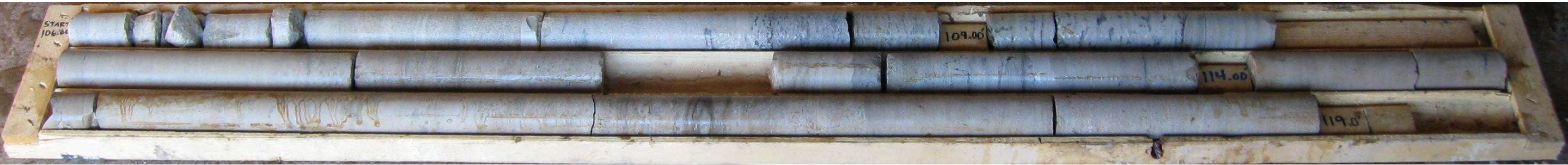
Photo 2: Borehole 102 – Rock Core. Elevation 154.58 metres to 150.28 metres.
