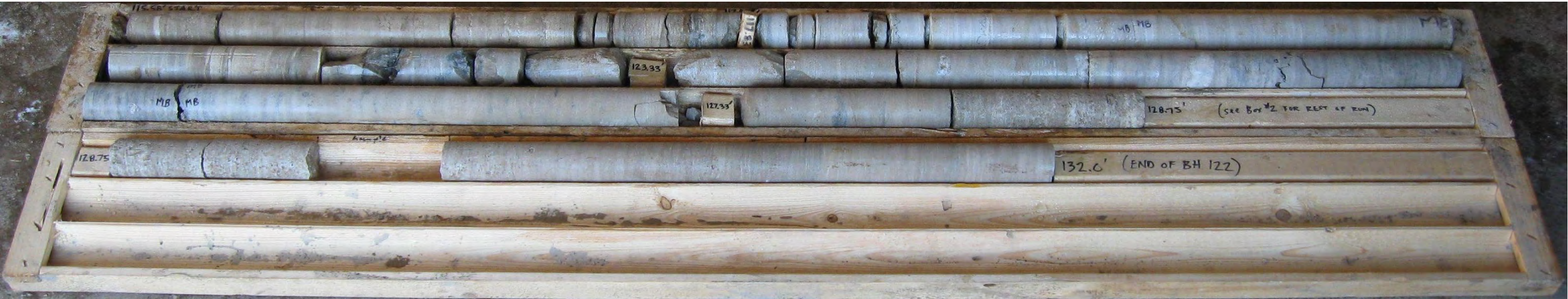
Photo 13: Borehole No. 122 – Rock Core. Elevation 146.61 metres to 141.33 metres.
