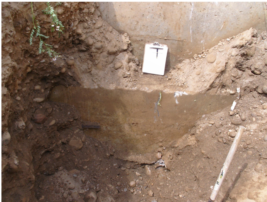
Photo 4: North Abutment Footing – East Side (Test Pit 102).
