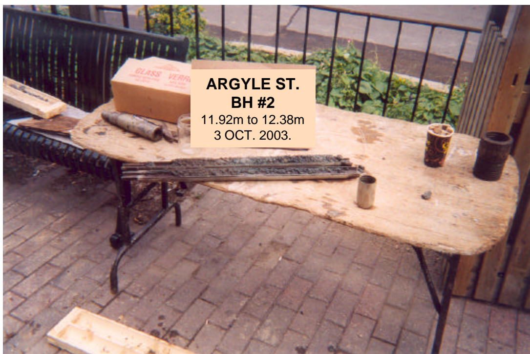
Photo 2 Borehole No. 2 – Split spoon in rock Elevation 178.31m to 177.85m.
