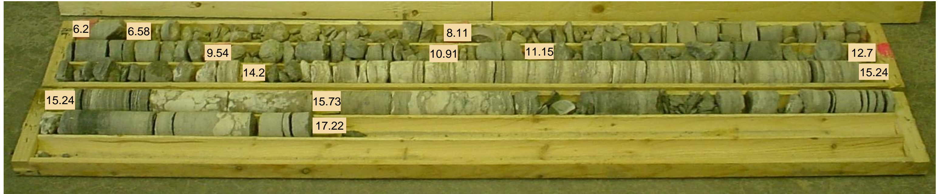
Photo 5: Borehole No. 101 – Rock Core. Possible concrete to approximate elevation 184.0 metres. Elevation 184.87 metres to 173.93 metres.
