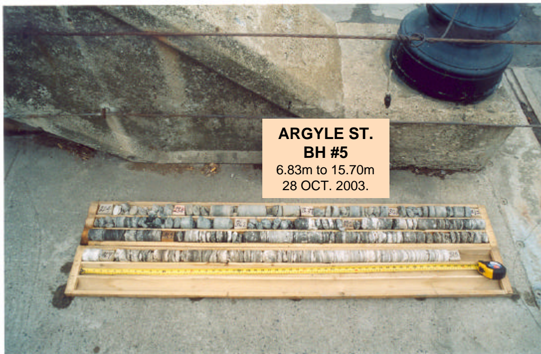
Photo 3 Borehole No. 5 – Rock core Elevation 184.59m to 175.72m.
