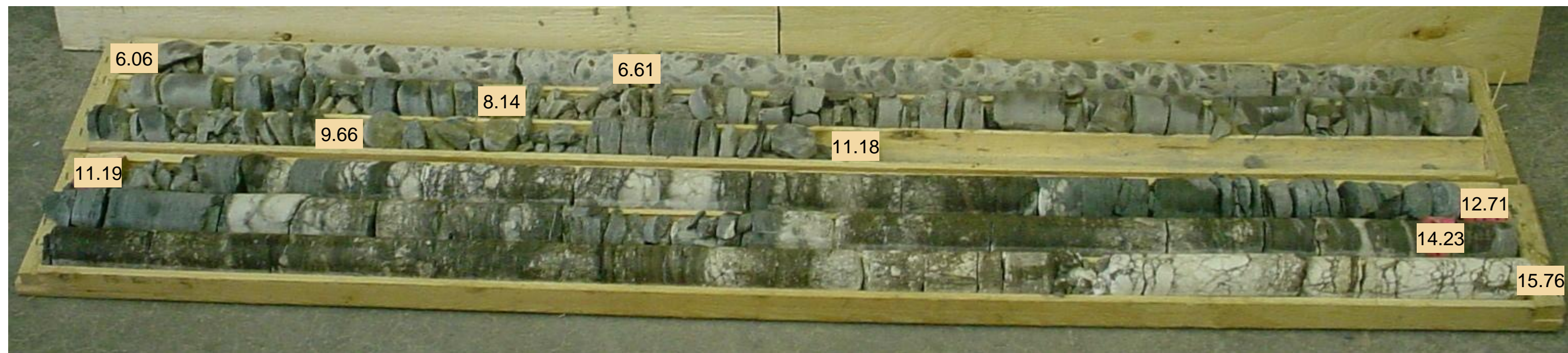
Photo 9: Borehole No. 105 – Rock Core. Concrete to approximate elevation 183.8 metres. Elevation 185.27 metres to 175.58 metres.
