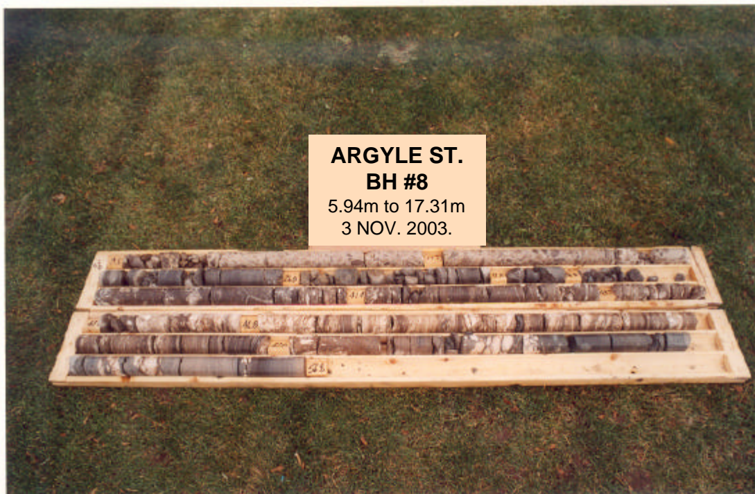
Photo 4 Borehole No. 8 – Rock core. Note concrete. Elevation 185.29m to 173.92m.
