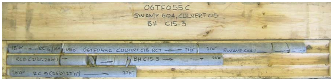
Photograph 11: Culvert at Sta. 13+206 (SBL and NBL) (C15), Cox Township, borehole C15-3. Cores 6 to 9 from 5.5 to 8.5 m depth. RQD values of 79 to 100%, indicating good to excellent rock quality.
