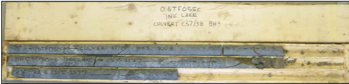
Photograph 13: Culvert at Sta. 15+279.1 (SBL and NBL) (C37/38), Cox Township, borehole C37/38-3. Cores 4 to 6 from 4.1 to 7.2 m depth. RQD values of 81 to 100%, indicating good to excellent rock quality.
