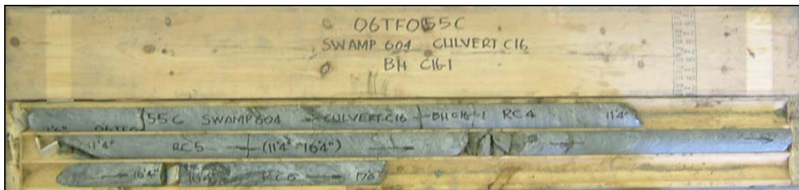
Photograph 12: Culvert at Sta. 8+240 (Crooked Lake Road South Connection) (C16), Cox Township, borehole C16-1. Cores 4 to 6 from 2.3 to 5.4 m depth. RQD values of 88 to 100%, indicating good to excellent rock quality.
