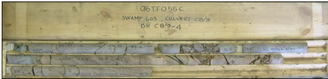
Photograph 9: Culvert at Sta. 12+590 (SBL and NBL) (C8/9), Cox Township, borehole C8/9-4. Cores 9 to 11 from 7.2 to 10.2 m depth. RQD values of 30 to 74%, indicating poor to fair rock quality.
