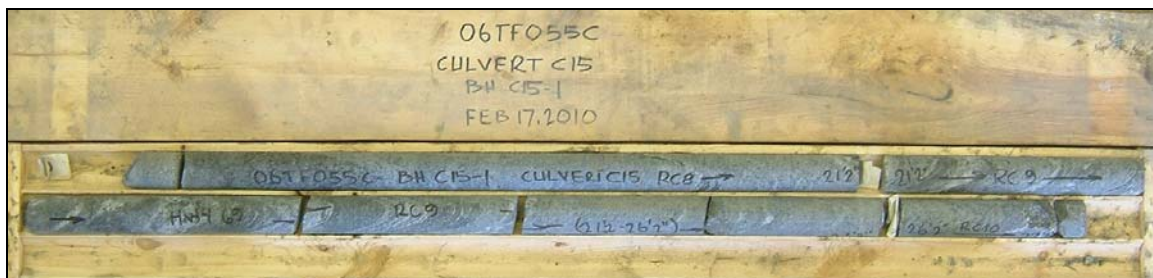
Photograph 10: Culvert at Sta. 13+206 (SBL and NBL) (C15), Cox Township, borehole C15-1. Cores 8 to 10 from 5.5 to 8.3 m depth. RQD values of 83 to 98%, indicating good to excellent rock quality.
