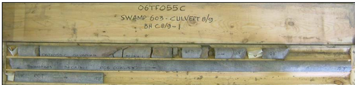
Photograph 8: Culvert at Sta. 12+590 (SBL and NBL) (C8/9), Cox Township, borehole C8/9-1. Cores 5 to 7 from 2.4 to 5.2 m depth. RQD values of 53 to 100%, indicating fair becoming excellent rock quality. Vertical fissures in the upper 0.7 m of the rock resulted in the lower rock quality.
