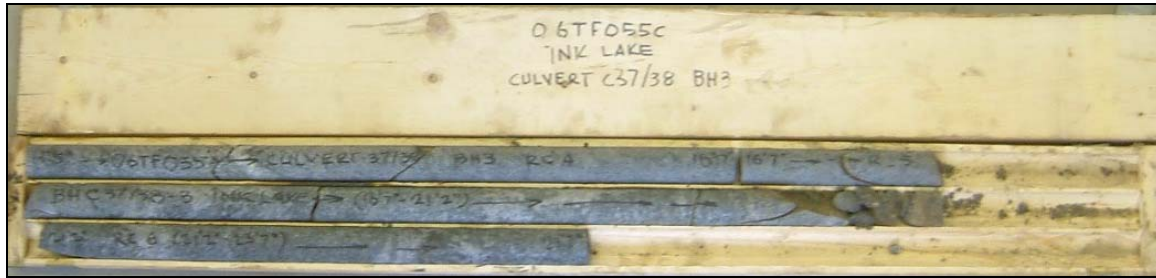
Photograph 13: Culvert at Sta. 15+279.1 (SBL and NBL) (C37/38), Cox Township, borehole C37/38-3. Cores 4 to 6 from 4.1 to 7.2 m depth. RQD values of 81 to 100%, indicating good to excellent rock quality.
