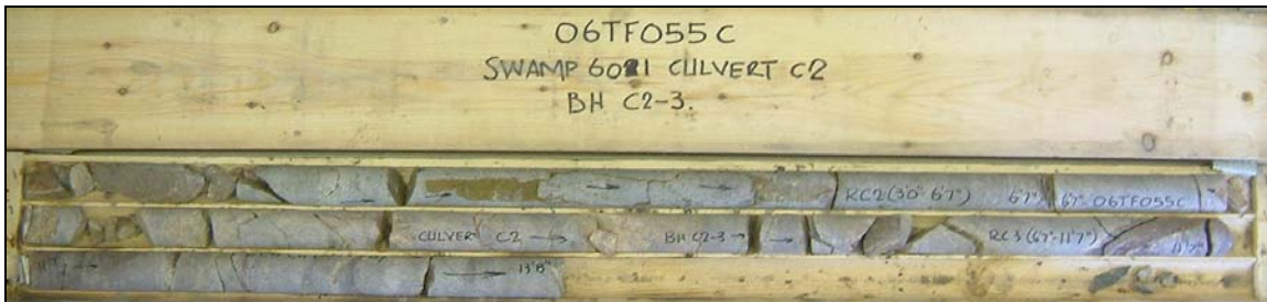
Photograph 4: Culvert at Sta. 10+140 (SBL) (C2), Cox Township, borehole C2-3. Cores 2 to 4 from 0.9 to 4.2 m depth. RQD values ranged from 33 to 80%, indicating poor to good rock quality.
