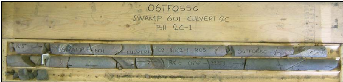
Photograph 3: Culvert at Sta. 10+140 (SBL) (C2), Cox Township, borehole C2-1. Cores 5 and 6 from 3.8 to 6.9 m depth. RQD values ranged from 50 to 52%, indicating fair rock quality.
