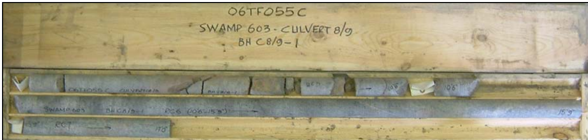
Photograph 8: Culvert at Sta. 12+590 (SBL and NBL) (C8/9), Cox Township, borehole C8/9-1. Cores 5 to 7 from 2.4 to 5.2 m depth. RQD values of 53 to 100%, indicating fair becoming excellent rock quality. Vertical fissures in the upper 0.7 m of the rock resulted in the lower rock quality.
