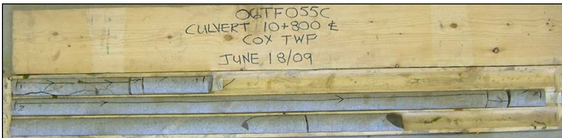
Photograph 6: Culvert at Sta. 10+800 (SBL and NBL) (SX), Cox Township, borehole SX-2. Cores 1 to 3 from 1.2 to 4.5 m depth. RQD values of 24 to 98%, indicating very poor to excellent rock quality.
