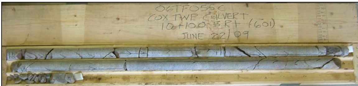
Photograph 2: Culvert at Sta. 10+100 (NBL) (C1), Cox Township, borehole C1-2. Cores 2 to 4 from 0.3 to 3.4 m depth. RQD values ranged from 40 to 79%, indicating poor to good rock quality.
