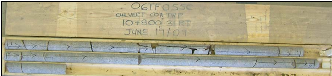
Photograph 7: Culvert at Sta. 10+800 (SBL and NBL) (SX), Cox Township, borehole SX-3. Cores 1 to 3 from 0.7 to 3.8 m depth. RQD values of 38 to 93%, indicating poor to excellent rock quality.
