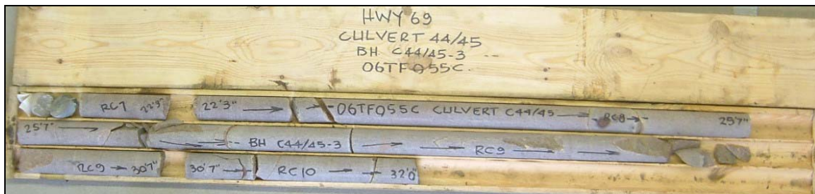
Photograph 16: Culvert at Sta. 10+523 (SBL) (C44), Servos Township, borehole C44/45-3. Cores 7 to 10 from 6.6 to 9.8 m depth. RQD values ranged from 83 to 100%, indicating good to excellent rock quality. Locally at 9.3 to 9.8 m depth, a RQD value of 41% was found indicating poor rock quality.
