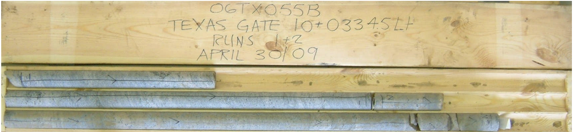
Photograph 3: Ungulate guard at Sta. 10+033.5, borehole 3, samples RC-4 and RC-5 from 1.9 to 4.9 m depth. The RQD values ranged from 92 to 100%, indicating excellent quality rock.
