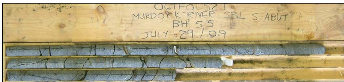
Photograph 2: Cores retrieved from borehole S5. Cores 3 to 5 from 2.1 to 5.2 m depth. RQD values ranged from 28 to 55%, indicating poor to fair rock quality.
