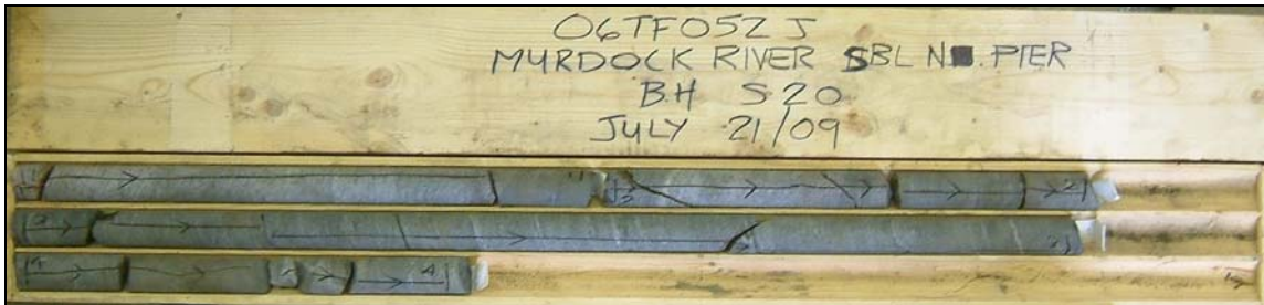
Photograph 10: Cores retrieved from borehole S20. Cores 1 to 4 from 0.0 to 3.1 m depth. RQD values ranged from 73 to 100%, indicating fair to excellent rock quality.
