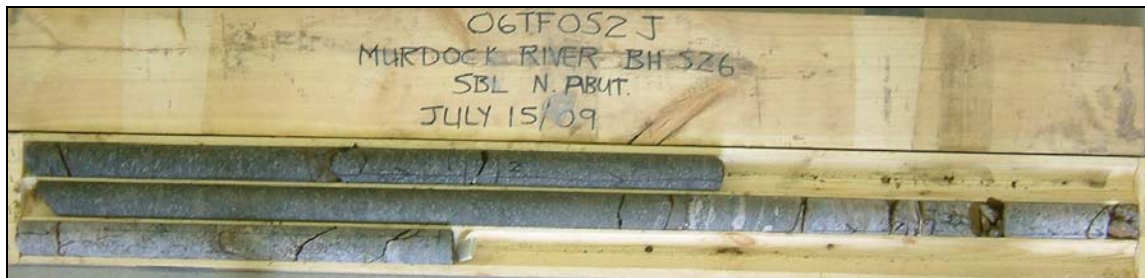
Photograph 14: Cores retrieved from borehole S26. Cores 2 to 4 from 1.2 to 4.4 m depth. RQD values ranged from 35 to 84%, indicating poor to good rock quality.
