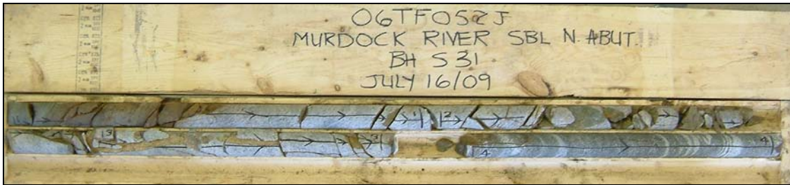
Photograph 17: Cores retrieved from borehole S31. Cores 5 to 8 from 4.1 to 7.0 m depth. RQD values ranged from 0 to 100%, indicating very poor to excellent rock quality.
