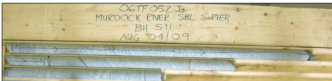
Photograph 6: Cores retrieved from borehole S11. Cores 1 and 2 from 0.3 to 3.4 m depth. RQD values of 99 and 100%, indicating excellent rock quality.
