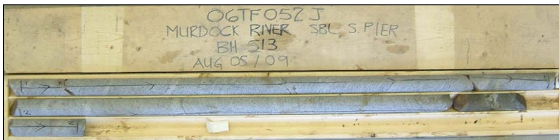
Photograph 7: Cores retrieved from borehole S13. Cores 1 and 2 from 0.0 to 3.2 m depth. RQD values of 94 and 98%, indicating excellent rock quality.
