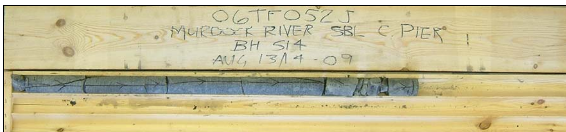
Photograph 8: Cores retrieved from borehole S14. Cores 8 and 9 from 14.0 to 15.3 m depth. RQD values of 52 and 80%, indicating fair to good rock quality.
