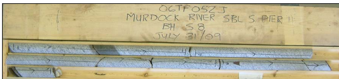
Photograph 4: Cores retrieved from borehole S8. Cores 3 to 5 from 1.2 to 4.3 m depth. RQD values ranged from 100 to 87%, indicating excellent becoming good rock quality.
