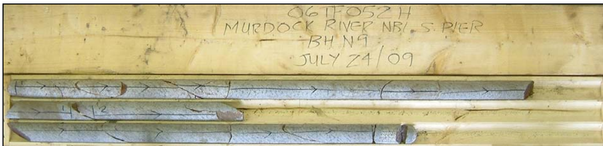
Photograph 5: Cores retrieved from borehole N9. Cores 1 and 2 from 0.0 to 3.1 m depth. RQD values of 86 and 87%, indicating good rock quality.
