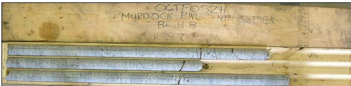
Photograph 4: Cores retrieved from borehole N8. Cores 1 to 4 from 0.3 to 3.5 m depth. RQD values ranged from 75 to 97%, indicating good to excellent rock quality.
