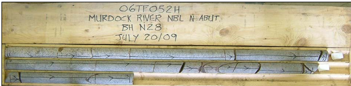
Photograph 14: Cores retrieved from borehole N28. Cores 1 to 3 from 0.0 to 3.4 m depth. RQD values ranged from 83 to 93%, indicating good to excellent rock quality.
