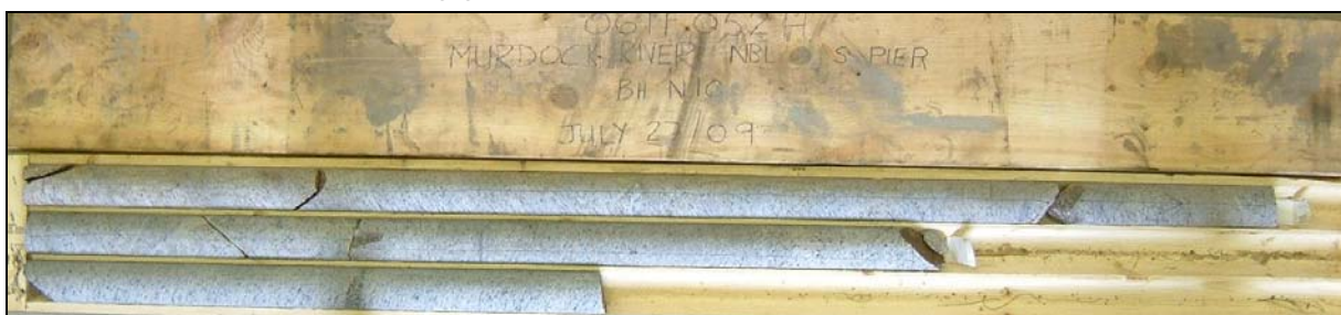
Photograph 6: Cores retrieved from borehole N10. Cores 1 to 3 from 0.0 to 3.2 m depth. RQD values ranged from 93 to 100%, indicating excellent rock quality.
