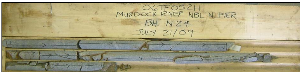
Photograph 10: Cores retrieved from borehole N24. Cores 1 to 3 from 0.4 to 3.5 m depth. RQD values ranged from 93 to 0%, indicating excellent becoming poor to very poor rock quality.
