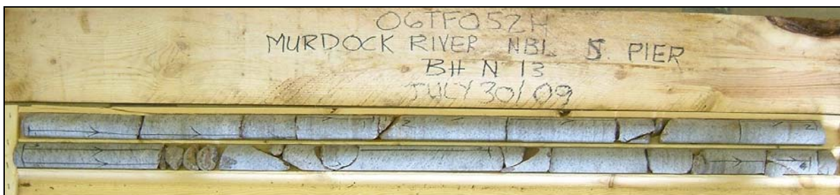
Photograph 7: Cores retrieved from borehole N13. Cores 1 to 4 from 0.0 to 3.1 m depth. RQD values ranged from 43 to 98%, indicating poor to excellent rock quality.
