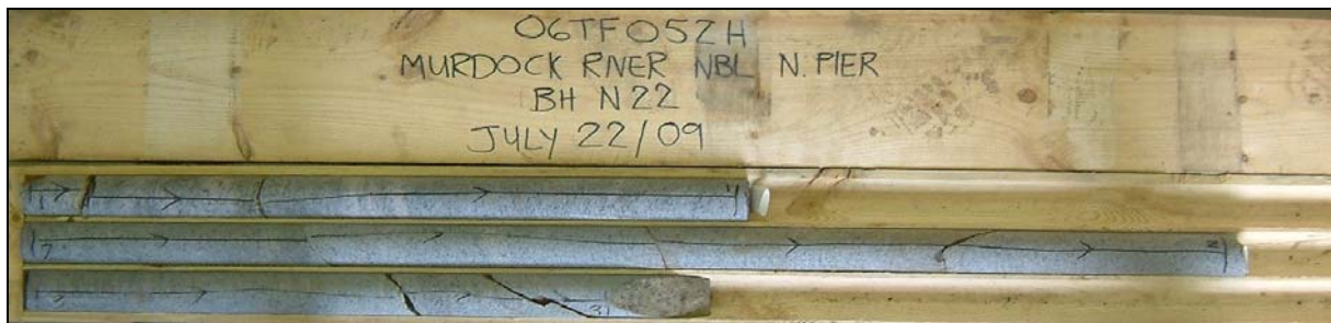
Photograph 9: Cores retrieved from borehole N22. Cores 3 to 5 from 1.2 to 4.4 m depth. RQD values ranged from 73 to 100%, indicating fair to excellent rock quality.
