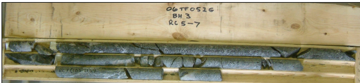
Photograph 1: Cores retrieved from borehole BH-3. Runs 5 to 7 from 4.1 to 7.1 m depth. RQD ranged from 76 to 100%. Good to excellent rock quality.
