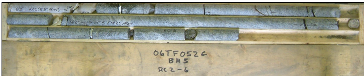
Photograph 3: Cores retrieved from borehole BH-5. Runs 4 to 6 from 3.3 to 6.5 m depth. RQD ranged from 81 to 100%. Good to excellent rock quality.
