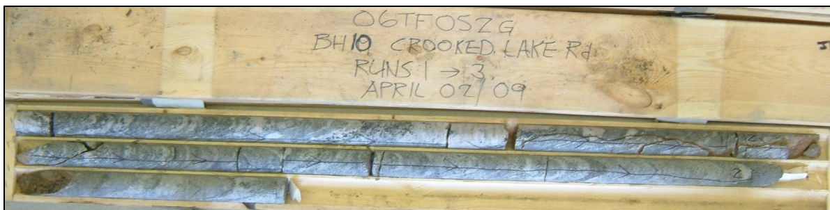
Photograph 6: Cores retrieved from borehole BH-10. Runs 1 to 3 from 0.2 to 3.5 m depth. RQD ranged from 97 to 100%, indicating excellent rock quality.
