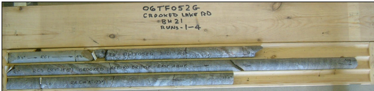
Photograph 13: Cores retrieved from borehole BH-21. Runs 2 to 4 from 2.3 to 5.3 m depth. RQD values obtained 94% for run 2 and 100% for runs 3 and 4, indicating excellent rock quality.
