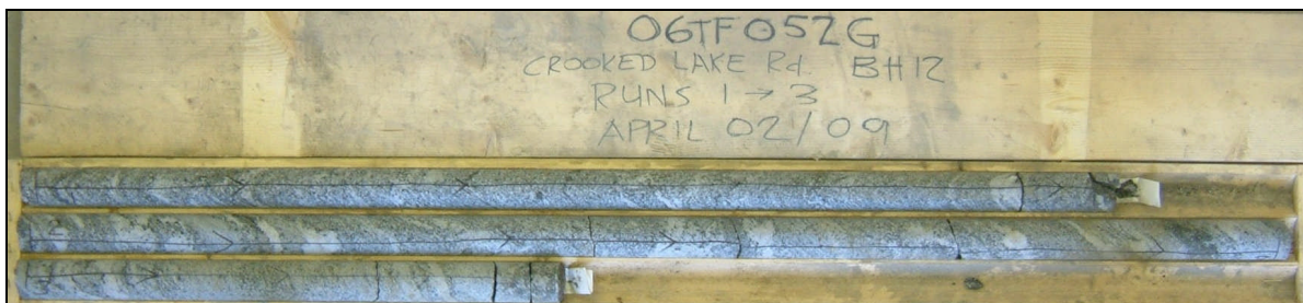
Photograph 8: Cores retrieved from borehole BH-12. Runs 1 to 3 from 0.0 to 3.5 m depth. RQD values obtained are 90 to 95%, indicating excellent rock quality.
