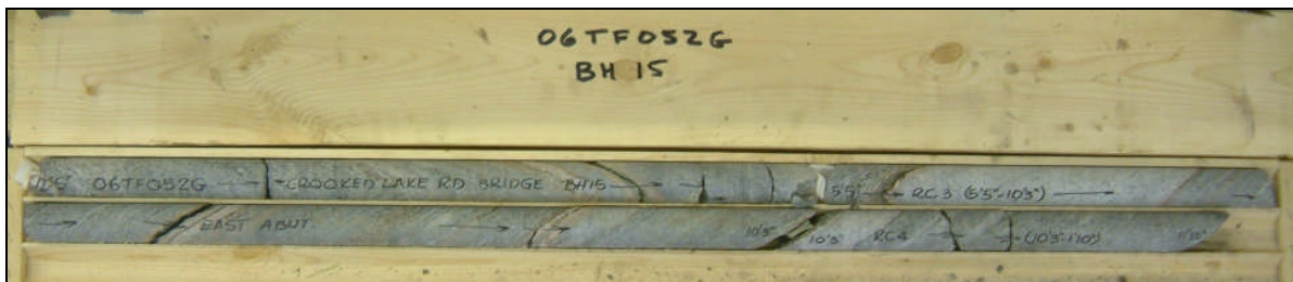
Photograph 9: Cores retrieved from borehole BH-15. Runs 2 to 4 from 0.7 to 3.6 m depth. RQD values obtained ranged from 82 to 100%, indicating good to excellent rock quality.
