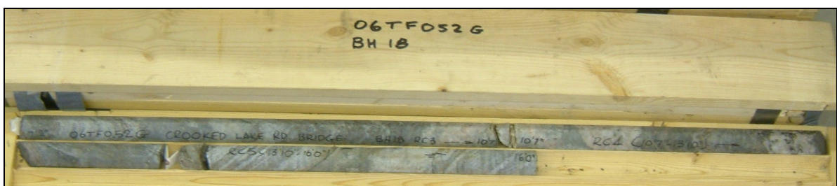
Photograph 12: Cores retrieved from borehole BH-18. Runs 3 to 5 from 2.2 to 4.9 m depth. RQD values obtained ranged from 80 to 97%, indicating good to excellent rock quality.
