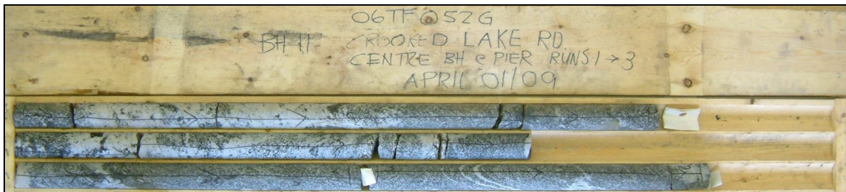
Photograph 7: Cores retrieved from borehole BH-11. Runs 1 to 3 from 0.0 to 3.4 m depth. RQD values obtained are 90 to 95%, indicating excellent rock quality.
