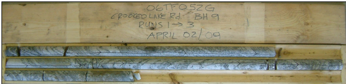
Photograph 5: Cores retrieved from borehole BH-9. Runs 1 to 3 from 0.1 to 3.4 m depth. RQD values obtained 97 to 100%, indicating excellent rock quality.
