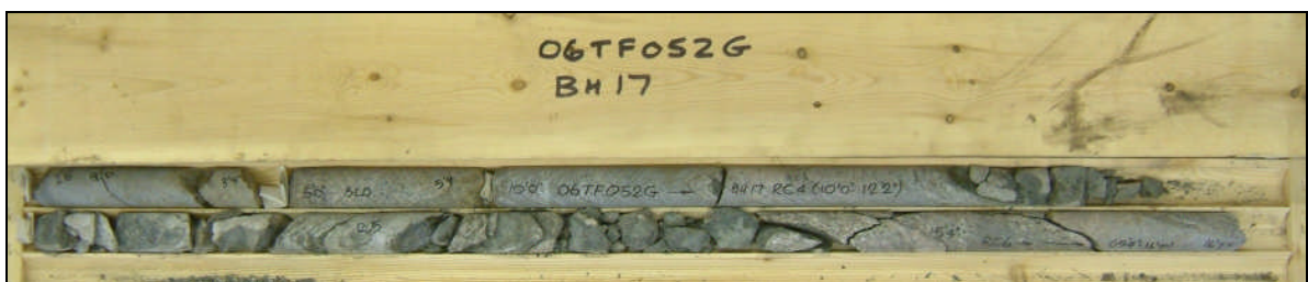
Photograph 11: Cores retrieved from borehole BH-17. Runs 4 to 6 from 3.0 to 5.1 m depth. RQD values obtained 79, 0 and 100% for runs 4, 5 and 6, respectively, indicating good to very poor becoming excellent rock quality.
