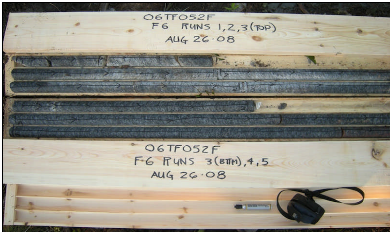
Photograph 5: Rock cores from borehole F6. Runs 1 and 5
