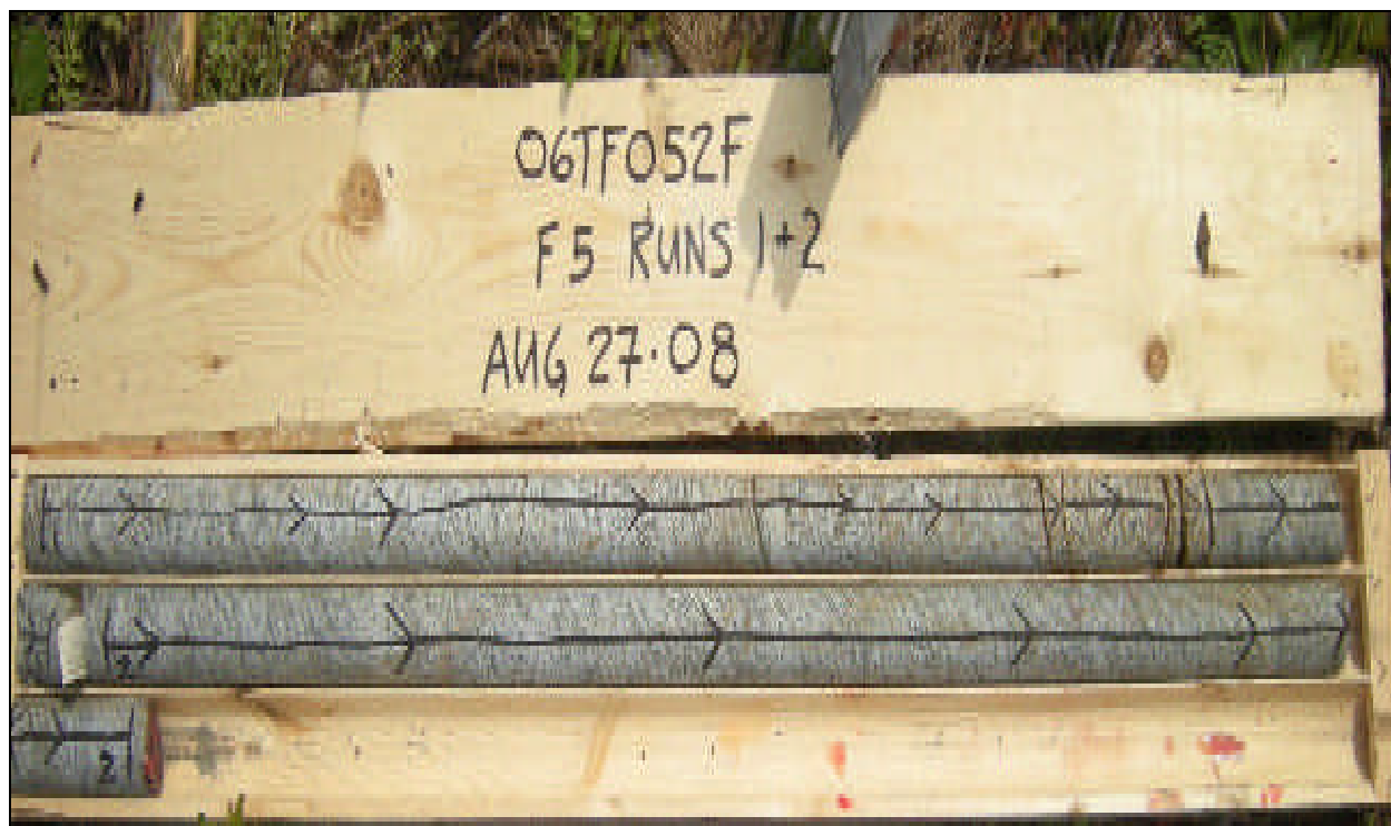
Photograph 4: Rock cores from borehole F5. Runs 1 and 2
