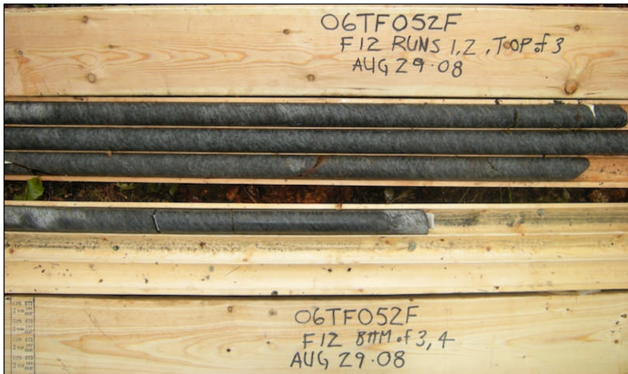
Photograph 11: Rock cores from borehole F12. Runs 1 to 4
