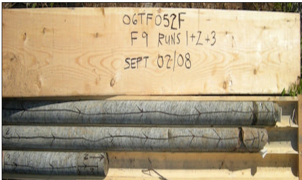
Photograph 8: Rock cores from borehole F9. Runs 1 to 3
