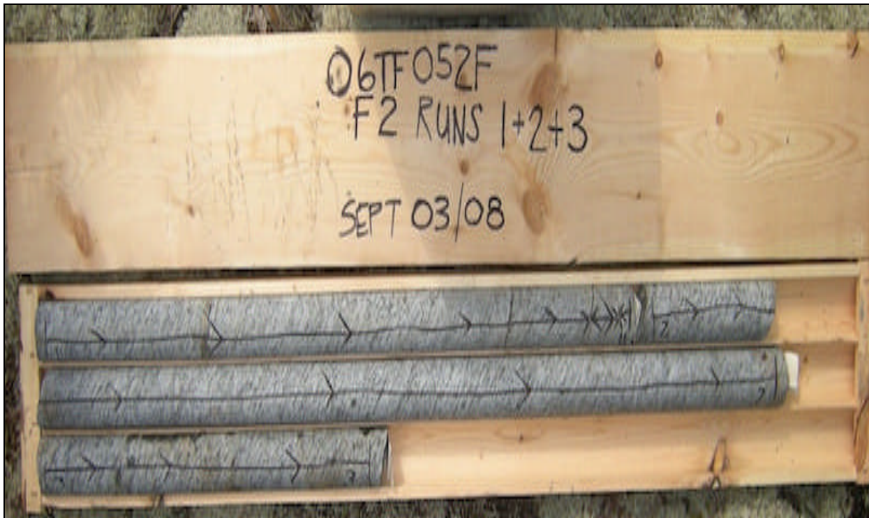
Photograph 1: Rock cores from borehole F2. Runs 1 to 3
