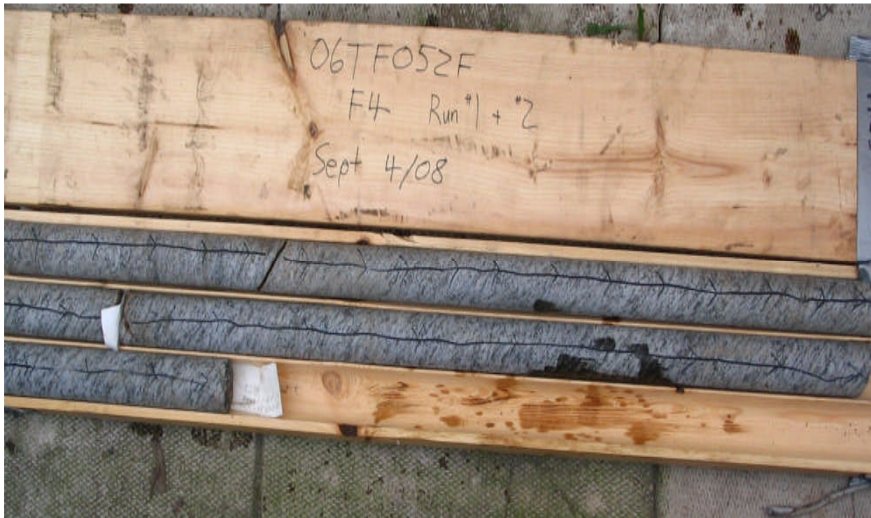
Photograph 3: Rock cores from borehole F4. Runs 1 and 2
