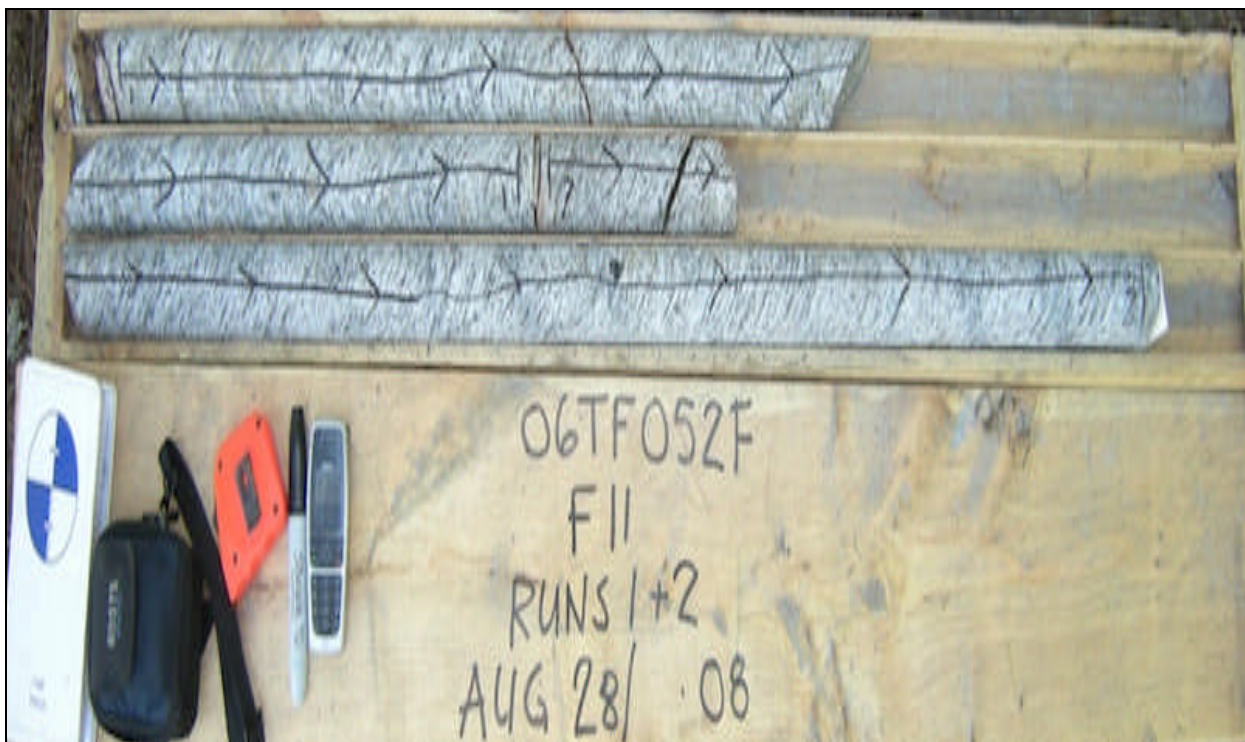
Photograph 10: Rock cores from borehole F11. Runs 1 and 2
