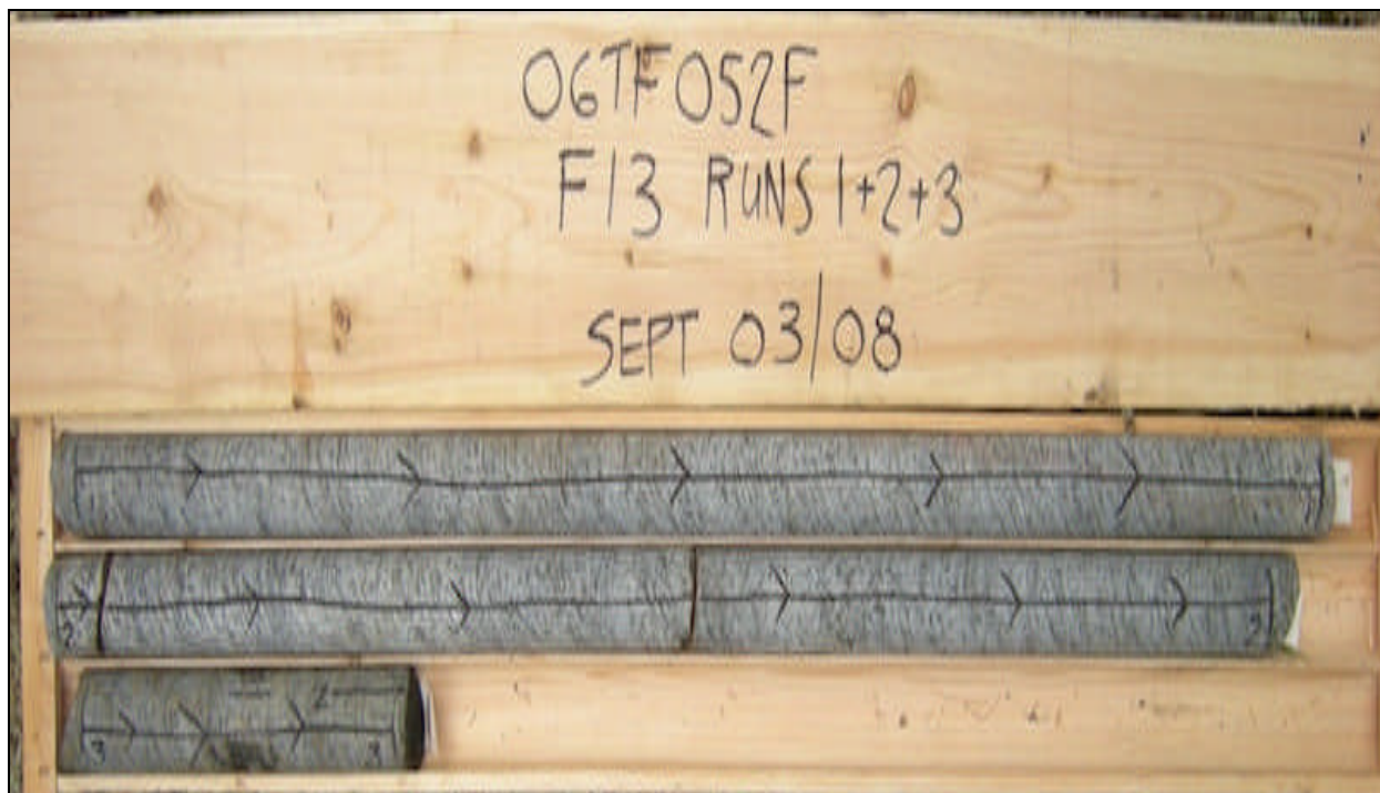
Photograph 12: Rock cores from borehole 13. Runs 1 to 3
