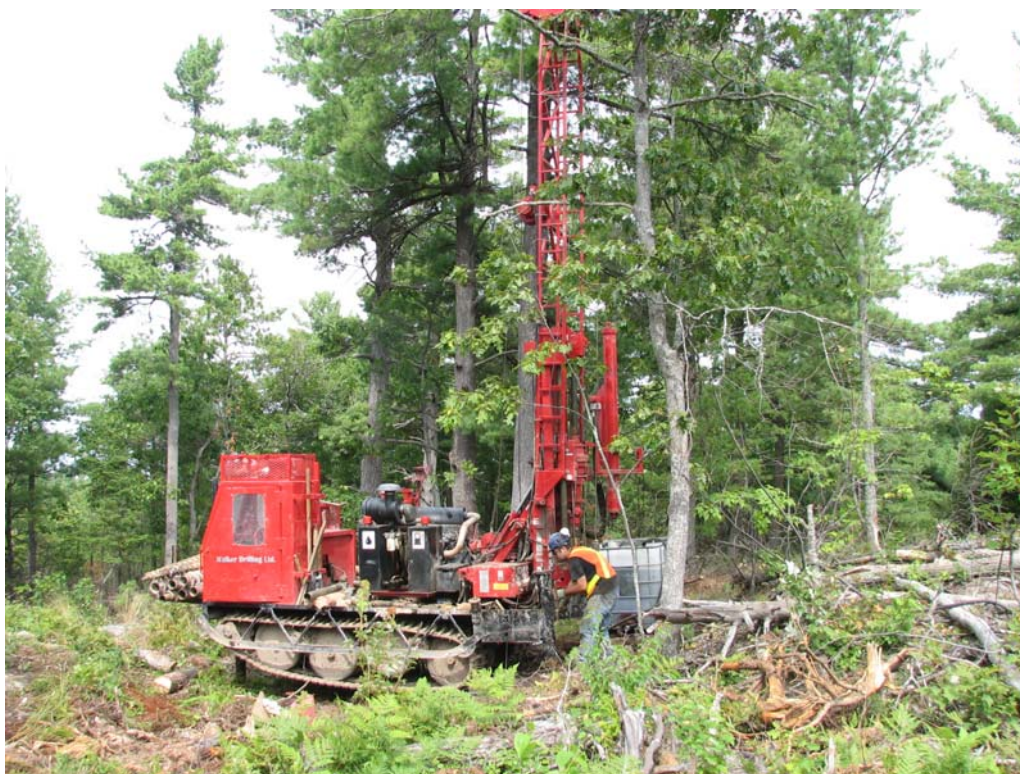
Image 3. Walker's Dietrich D 50 Turbo preparing to set up on hole F8.
