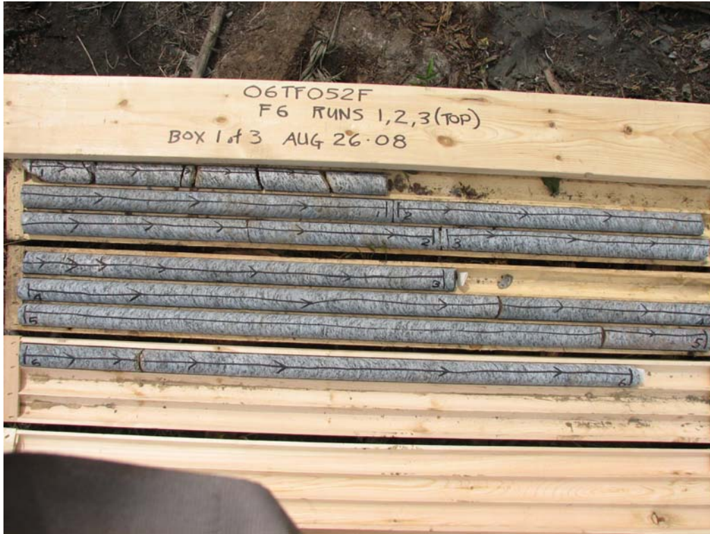
Image 5. Typical rock mass conditions encountered during drilling with very high quality rock mass with very few natural discontinuities, and very strongly developed metamorphic fabric.
