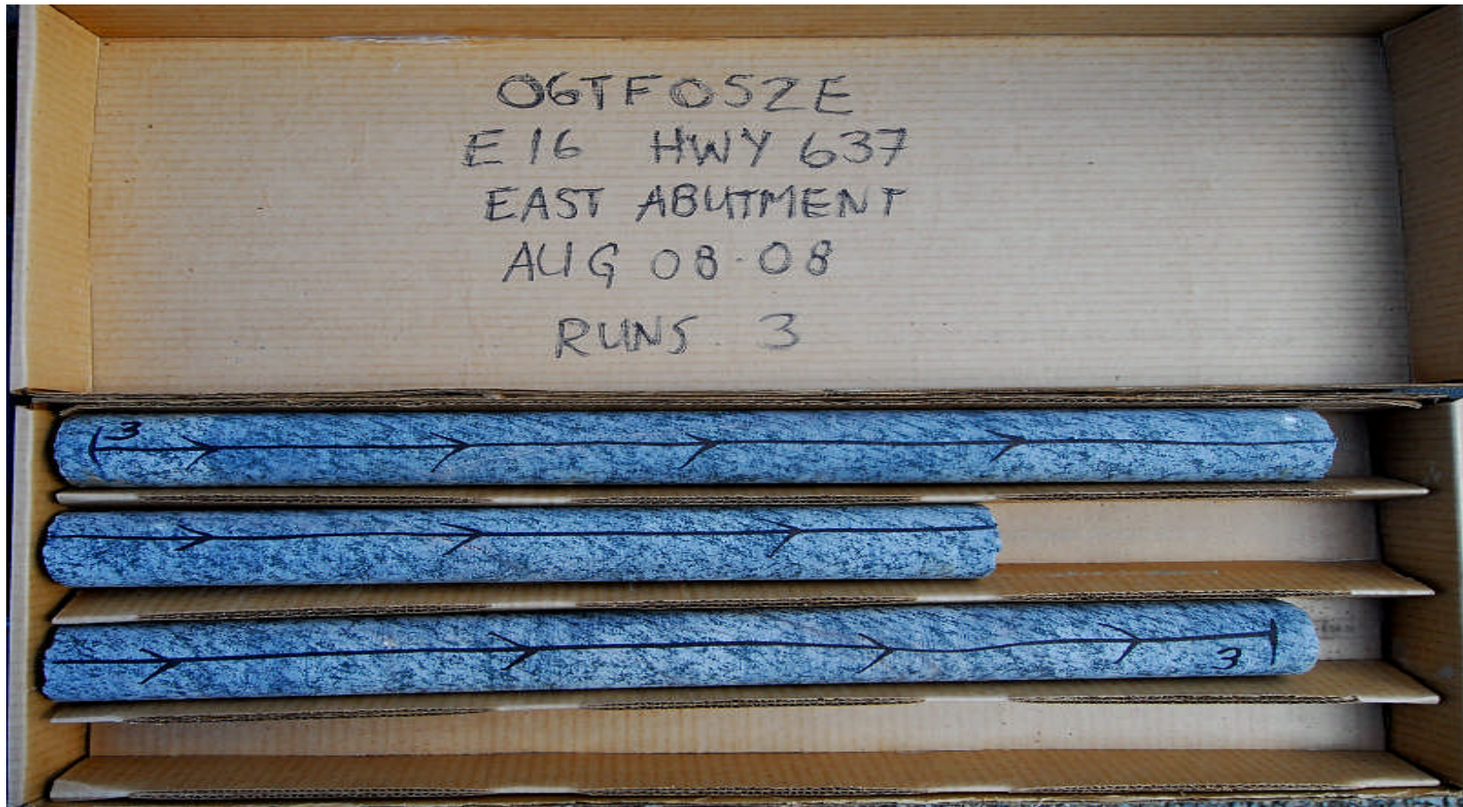
East Abutment Core Photograph 4: Rock core from borehole E16 - RC-7
