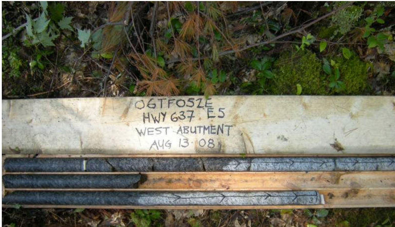
West Abutment Core Photograph 3: Rock core from borehole E5 - RC-1 to RC-3
