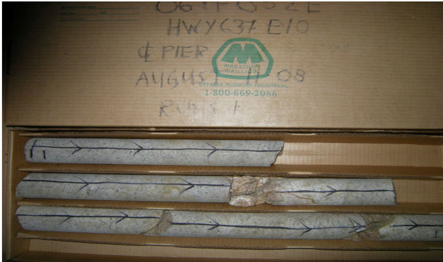
Centre Pier Core Photograph 2 : Rock core from borehole E10 - RC-1
