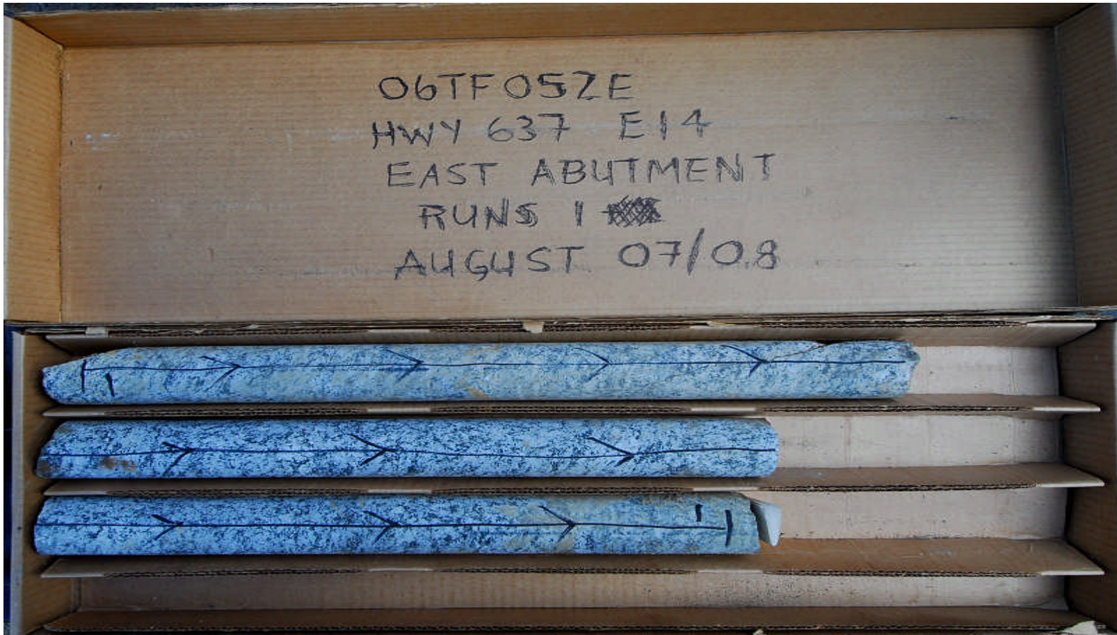
East Abutment Core Photograph 1: Rock core from borehole E14 - RC-2
