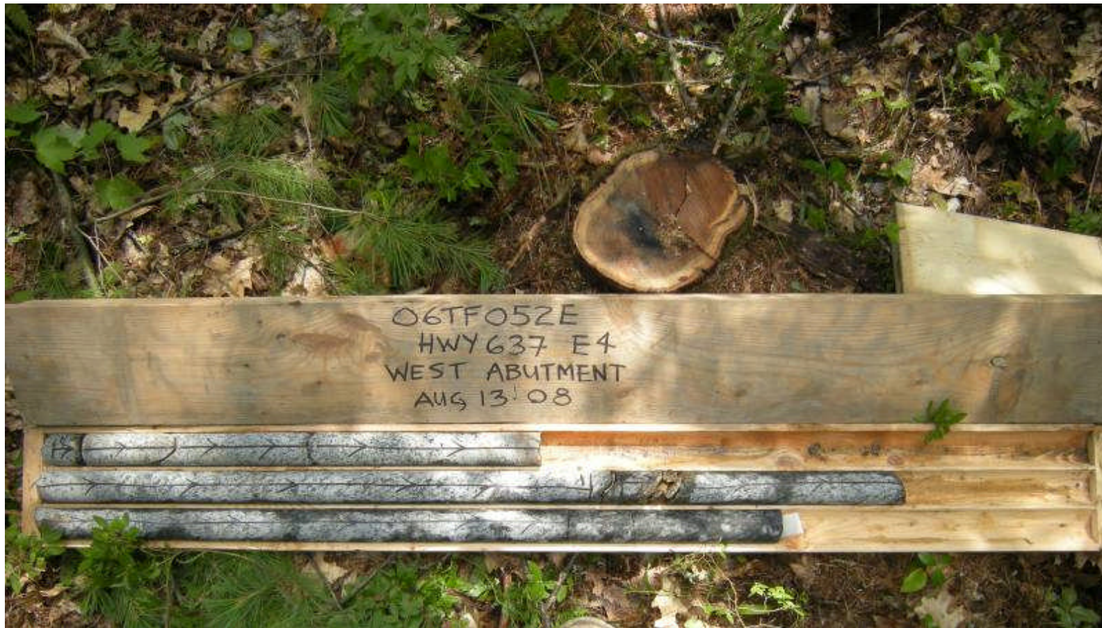
West Abutment Core Photograph 2 : Rock core from borehole E4 - RC-1 and RC-2
