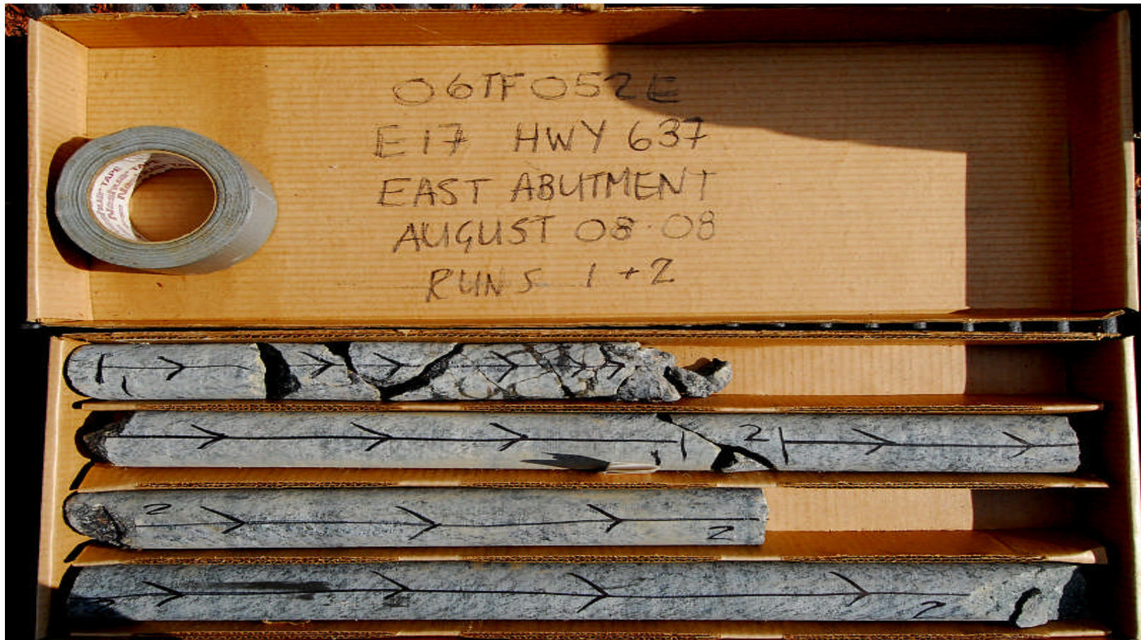
East Abutment Core Photograph 5: Rock core from borehole E17 - RC-5 and top of RC-6
