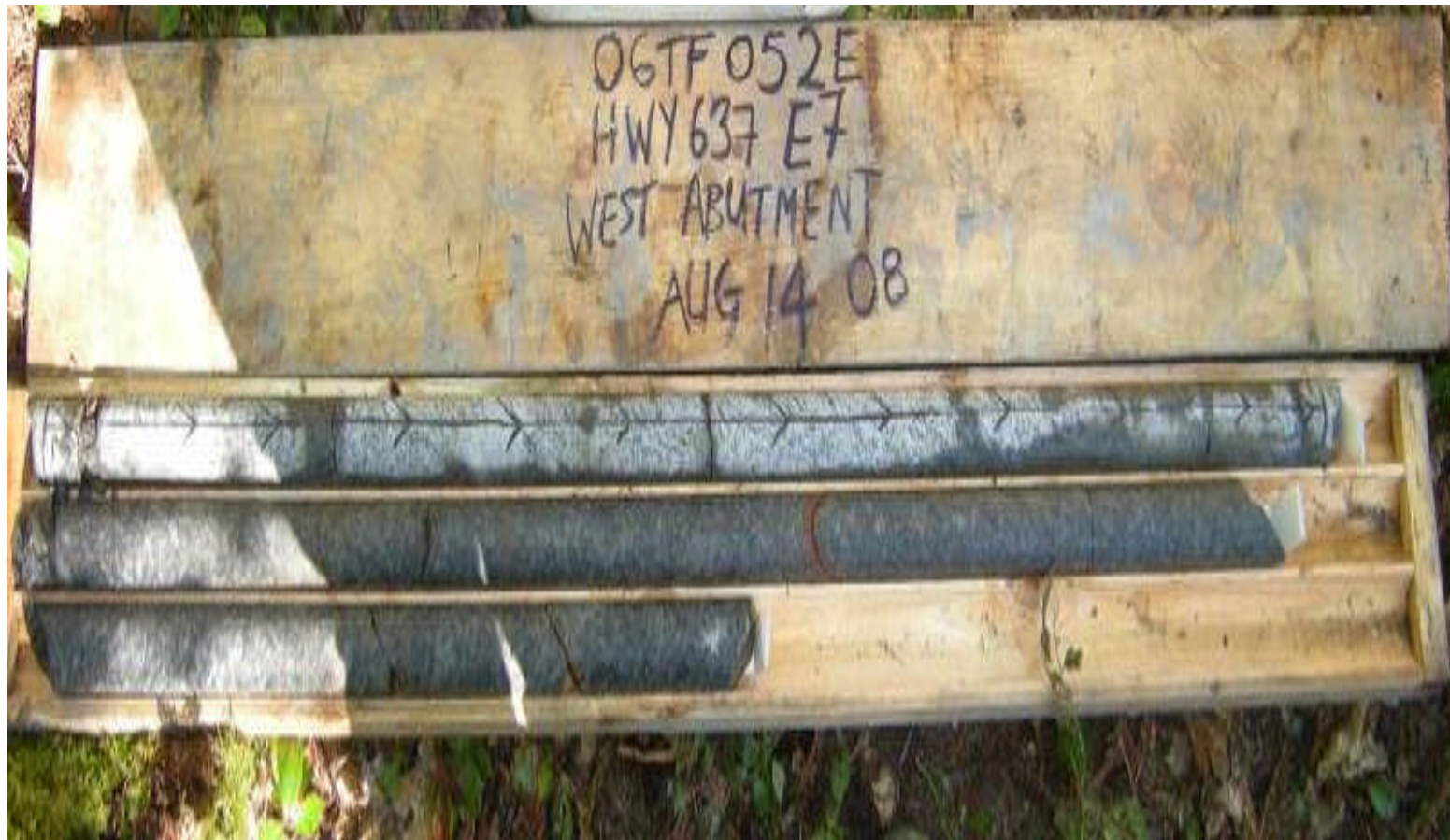
West Abutment Core Photograph 4: Rock core from borehole E7 - RC-1, RC-2 and RC-3
