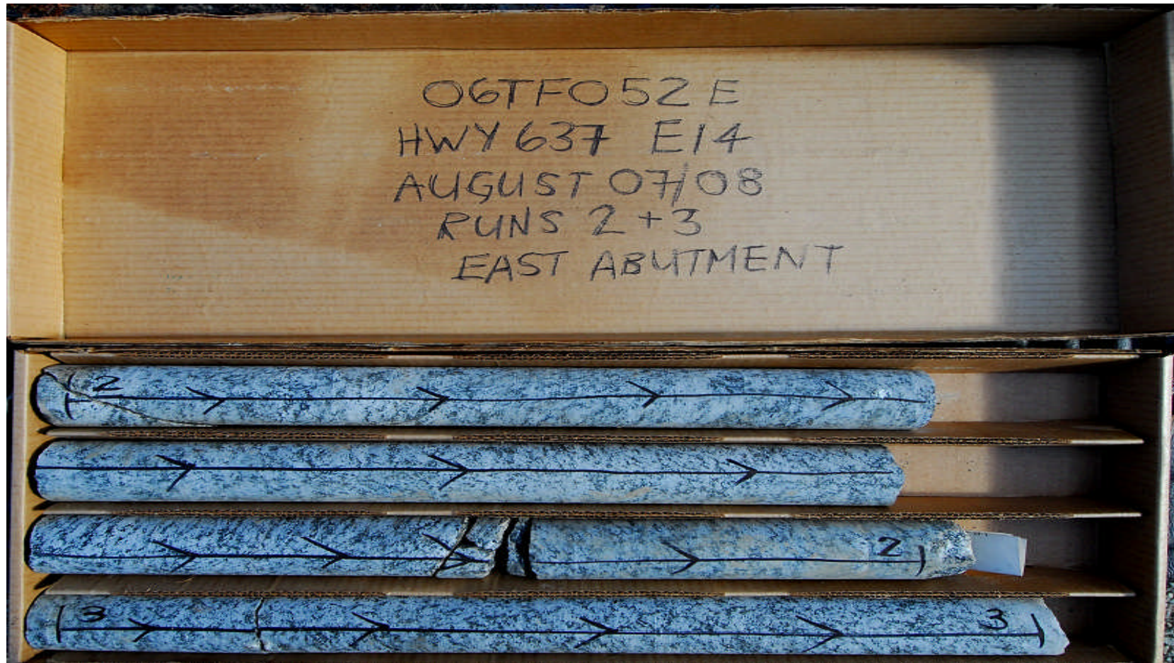
East Abutment Core Photograph 2: Rock core from borehole E14 - RC-3 and RC-4
