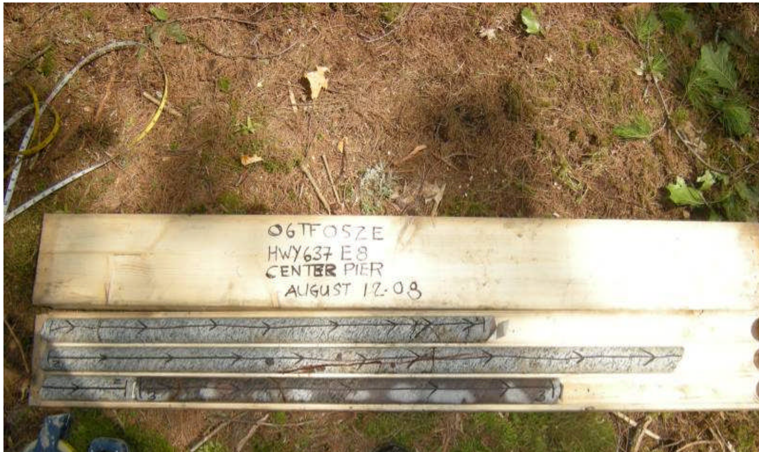
Centre Pier Core Photograph 1 : Rock core from borehole E8 - RC-1, RC-2 and RC-3
