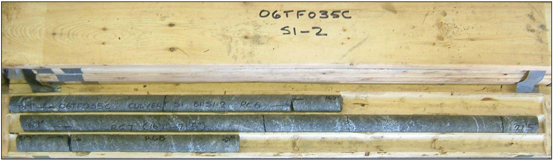
Photograph 1: Culvert S1, borehole S1-1, samples RC-8 to RC-10 from 6.9 to 9.9 m depth. The RQD values ranged from 98 to 100%, indicating excellent quality bedrock.
