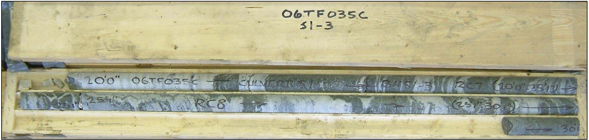
Photograph 3: Culvert S1, borehole S1-3, samples RC-7 and RC-8 from 6.1 to 9.2 m depth. The RQD values were 100%, indicating excellent quality bedrock.
