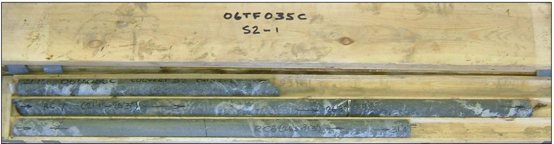
Photograph 4: Culvert S2, borehole S2-1, samples RC-7 and RC-8 from 6.4 to 9.5 m depth. The RQD values were 100%, indicating excellent quality bedrock.
