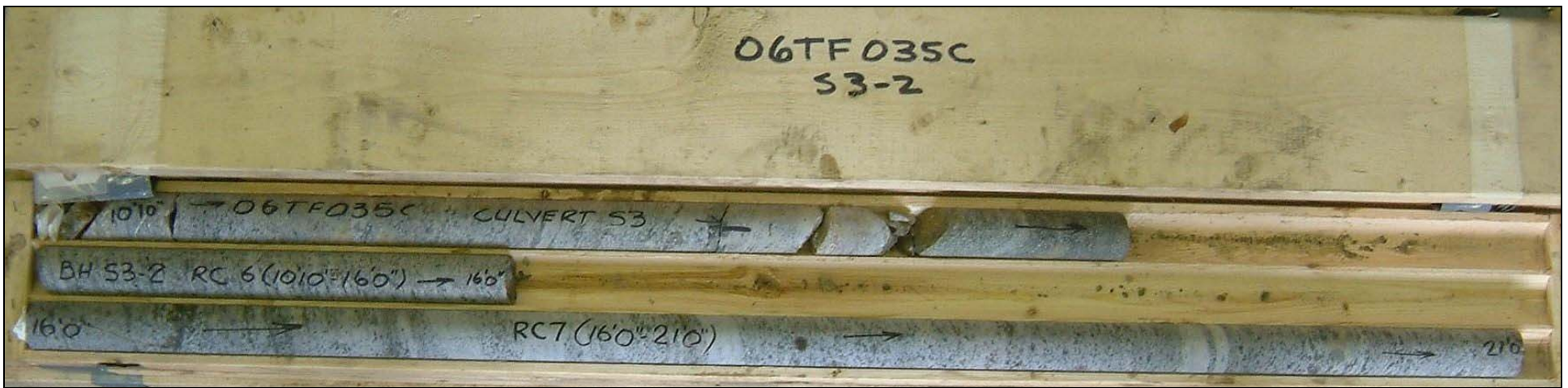
Photograph 8: Culvert S3, borehole S3-2, samples RC-6 and RC-7 from 3.3 to 6.4 m depth. The RQD values ranged from 85 to 97%, indicating good to excellent quality bedrock.
