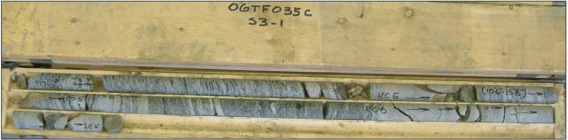
Photograph 7: Culvert S3, borehole S3-1, samples RC-5 and RC-6 from 3.2 to 6.2 m depth. The RQD values ranged from 35 to 100%. The Granitic Gneiss bedrock contacted from 3.2 to 4.7 m depth was good quality, the Migmatite bedrock contacted from 4.7 to 5.4 m depth was excellent quality and the Arkose bedrock contacted at 5.4 to 6.2 m depth was poor quality.
