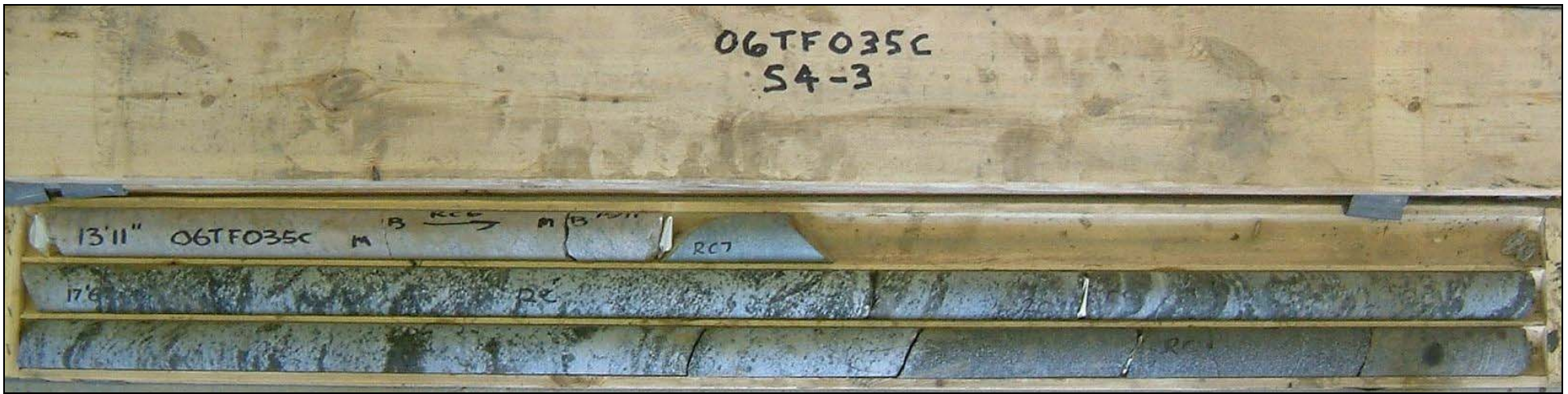
Photograph 12: Culvert S4, borehole S4-3, samples RC-6 to RC-9 from 4.2 to 8.3 m depth. The RQD values ranged from 98 to 100%, indicating excellent quality bedrock. Cobbles and boulders were contacted to 5.3 m depth.
